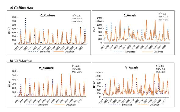
**Figure 4.** Observed and simulated stream-flow  $(10^6 \text{ m}^3)$  at selected stations in the Upper Awash Basin: (a) Calibration, and (b) validation.
