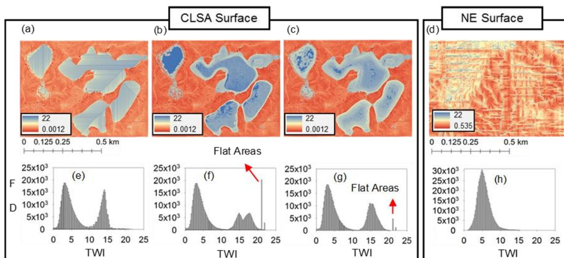
**Figure 5.** Visual comparisons of topographic wetness index (TWI) computations (a–d) and frequency distributions (FD) (e–h) for two different surfaces: depression-dominated Cottonwood Lake Study Area (CLSA) surface (a–c) and dendritic Nelson Eddy (NE) surface (d); TWI values were calculated for the CLSA surface based on (a) filled DEM; (b) original DEM; and (c) corrected DEM.
