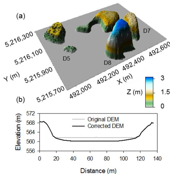
**Figure 4.** (a) 3D distribution of the elevation differences between the original digital elevation model (DEM) and the corrected DEM that incorporates the pothole bathymetry data; (b) comparison between the two DEMs for a cross-section of depression D7.
