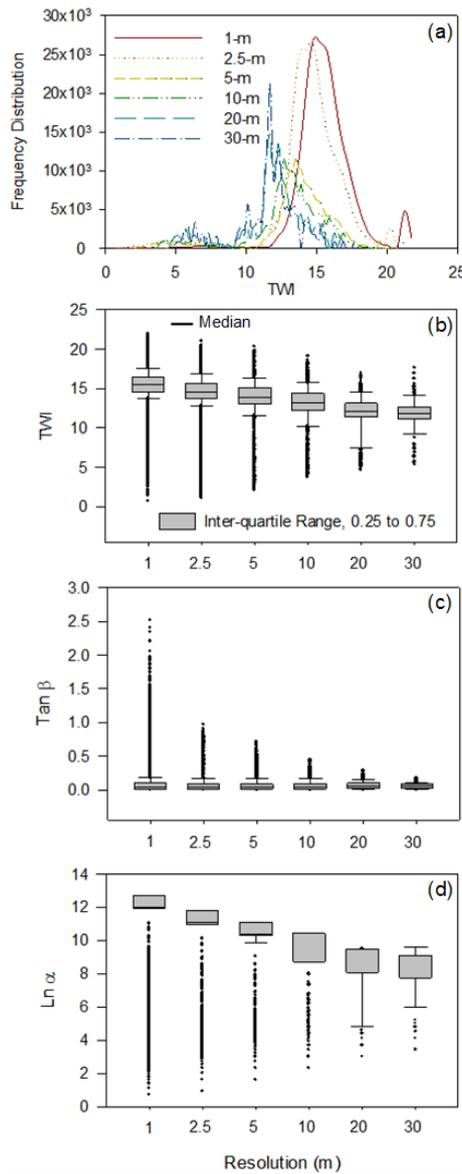
**Figure 7.** Frequency distribution of TWI (a) and statistical summary of TWI (b),  $\tan(\beta)$  (c), and  $\ln(\alpha)$  (d) for 1-m, 2.5-m, 5-m, 10-m, 20-m, and 30-m resolutions of depressional grids on the Cottonwood Lake Study Area (CLSA) surface using the modified TWI procedure.
