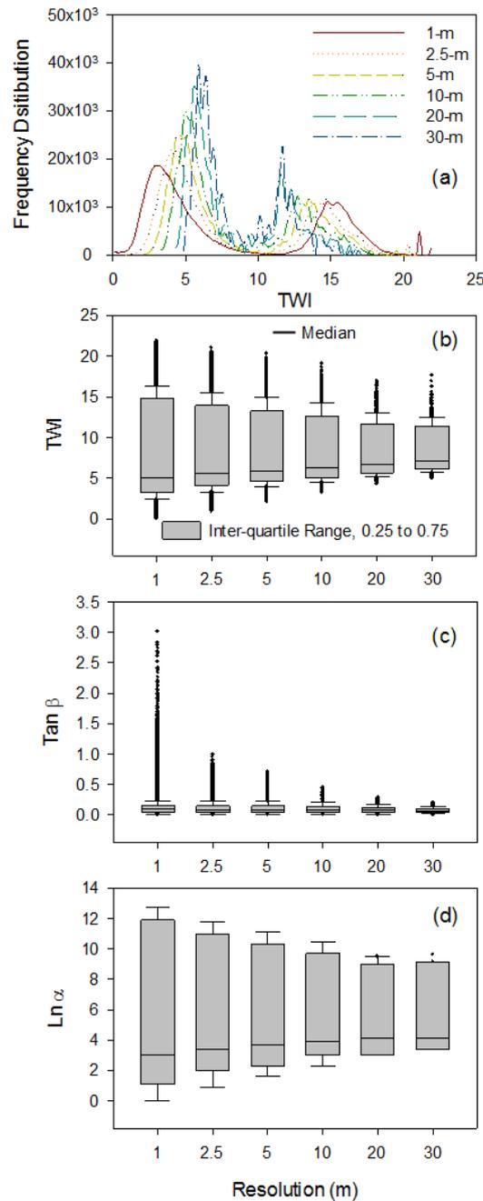
**Figure 6.** Frequency distribution of TWI (a) and statistical summary of TWI (b),  $\tan(\beta)$  (c), and  $\ln(\alpha)$  (d) for 1-m, 2.5-m, 5-m, 10-m, 20-m, and 30-m resolutions of the entire Cottonwood Lake Study Area (CLSA) surface using the modified TWI procedure.
