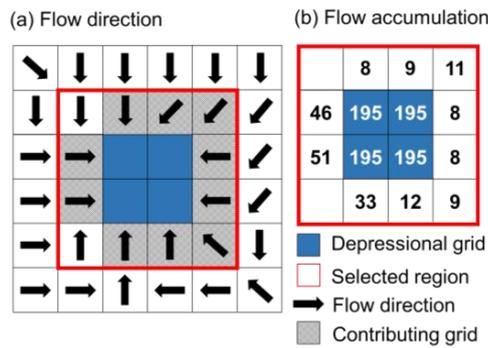
**Figure 3.** Schematic representation of (a) flow direction and (b) flow accumulation for a depression/puddle.
