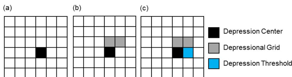
**Figure 2.** Identification of depressional elements in the puddle delineation (PD) algorithm: (a) center grid; (b) depressional grids; and (c) threshold grid.
