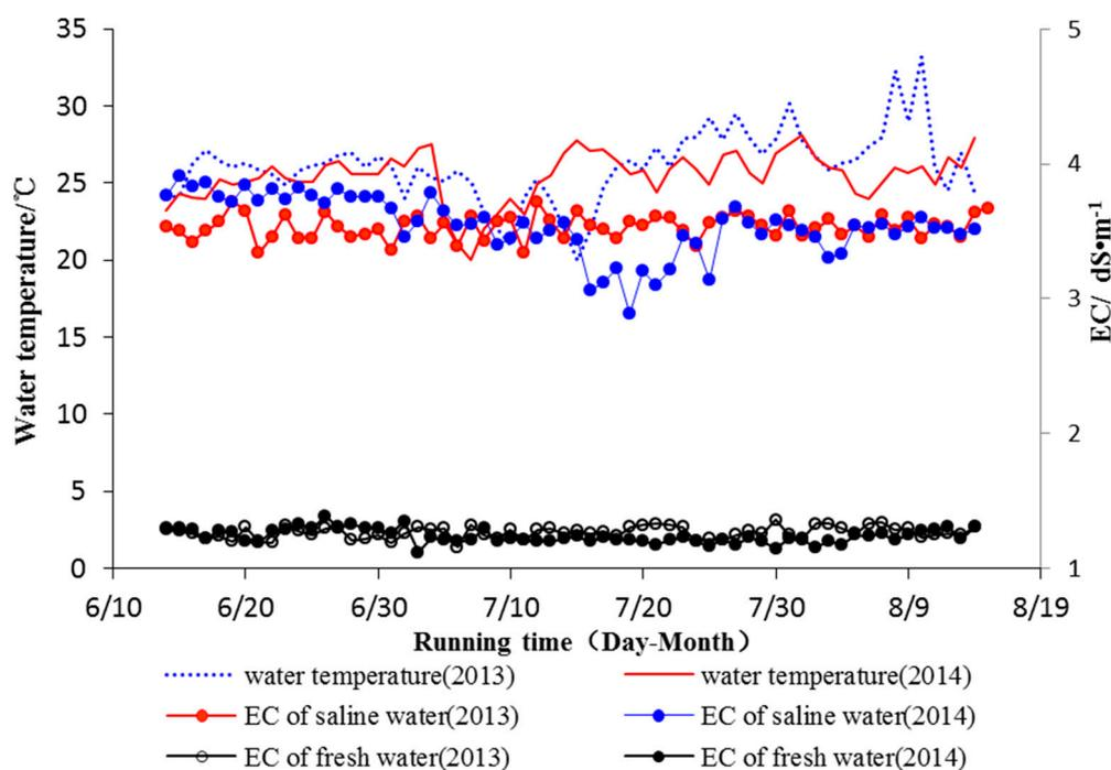
**Figure 2.** Variation in water temperature and electrical conductivity (EC) during the experiment.
