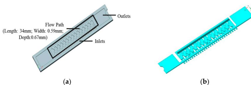
**Figure 1.** Three-dimensional (3D) structure (a) and inner flow field (b) of the drip irrigation emitter.
