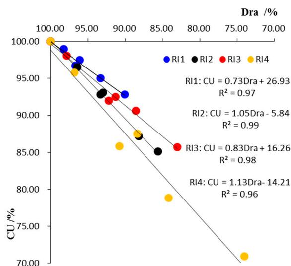
Figure 5. Relationship between Dra and CU under different fresh-saline alternating irrigation models.
