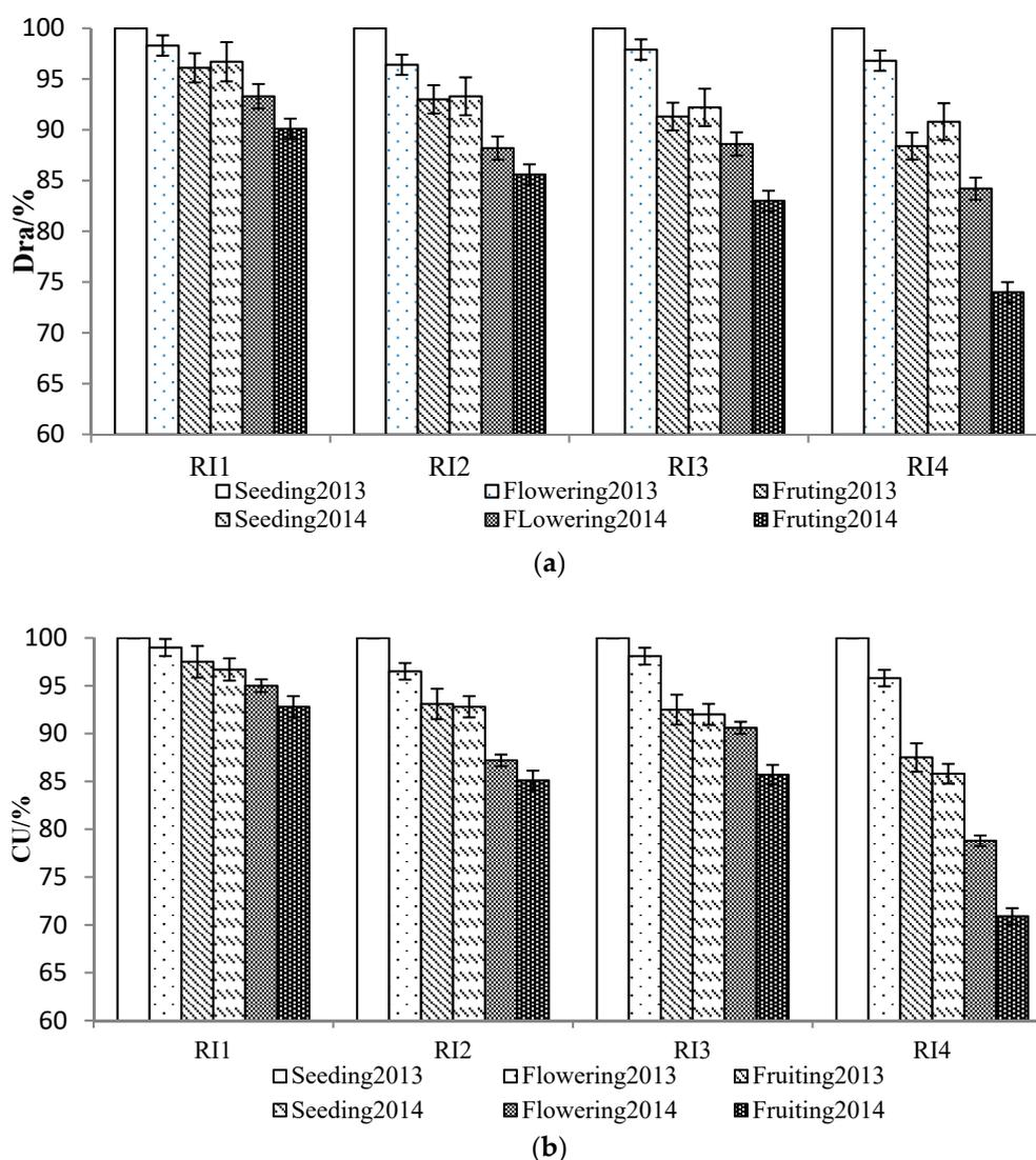
**Figure 3.** Discharge ratio variation (Dra) (a) and Christiansen coefficient of uniformity (CU) (b) variation under different fresh-saline alternating irrigation model.
