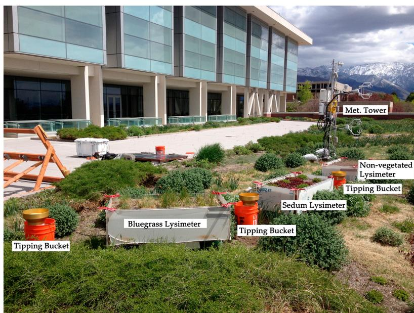
Figure 2. Photograph of the experimental setup.
