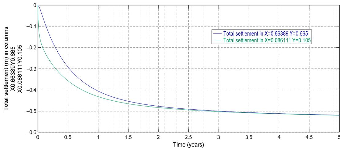
Figure 19. Surface settlement evolution in two soil columns. (a = b = 0.7 m; c = 0.05 m; d = 4 m).
