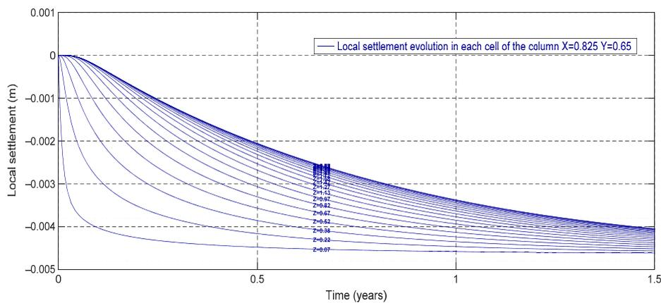
Figure 13. Evolution of the local settlement in each of the cells of a soil column ( $N_z = 20$ ).
