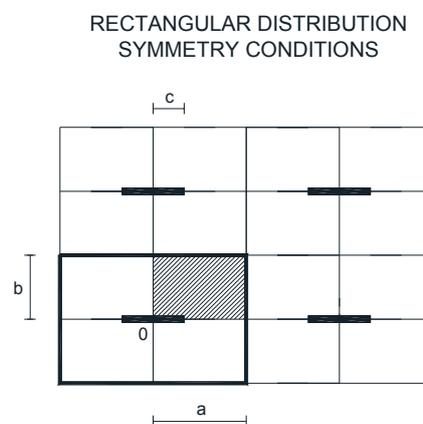
**Figure 2.** Symmetry conditions of the rectangular layout.
