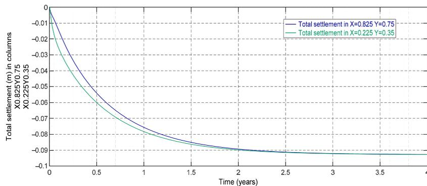
Figure 14. Surface settlement evolution of two soil columns.
