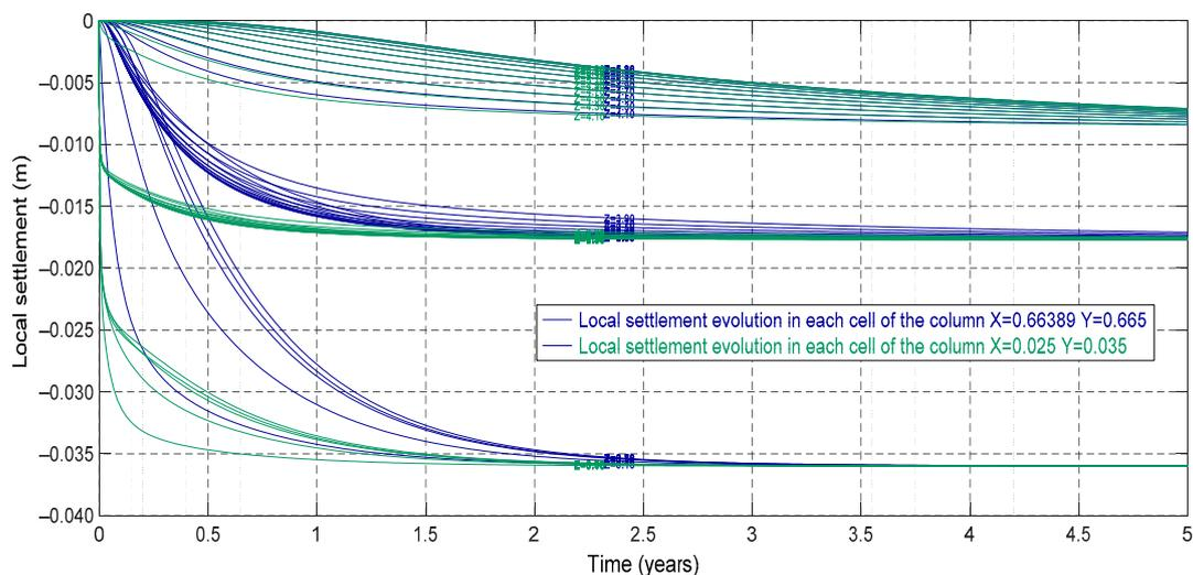
**Figure 18.** Local settlement evolution in each of the cells of two soil columns. ( $a = b = 0.7\text{ m}$ ;  $c = 0.05\text{ m}$ ;  $d = 4\text{ m}$ ).
