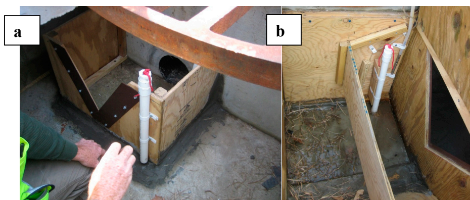
Figure 5. (a) Sixty-degree v-notch weir installed to measure drainage from the underdrain and pond water for sampling (flow direction from background to foreground); (b) Ninety-degree v-notch weir installed to measure overflow/bypass with a baffle (center) to still flow for sampling (flow direction from left to right).
