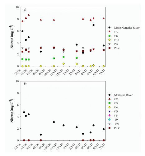
**Figure 1.** Nitrate (in NO<sub>3</sub>–N) in (**a**) Auburn and (**b**) Nebraska City. LNR: Little Nemaha River; MR: Missouri River; Pre: Inflow water to the water treatment plants prior to any additional treatment; Post: Water collected at the two water treatment plants after chlorination.
