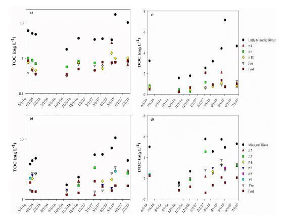
**Figure 2.** Total organic carbon (TOC) in (**a**) Auburn and (**b**) Nebraska City and dissolved organic carbon (DOC) in (**c**) Auburn and (**d**) Nebraska City. LNR: Little Nemaha River; MR: Missouri River; Pre: Inflow water to the water treatment plant prior to any additional treatment; Post: Water collected at the two water treatment plants after chlorination.
