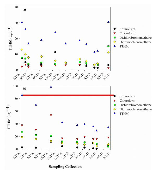
**Figure 3.** Total Trihalomethanes (TTHM) in (**a**) Auburn and (**b**) Nebraska City. Water samples were collected at the two water treatment plants after chlorination. Total TTHM maximum contaminant level (MCL): 80  $\mu$ g L<sup>-1</sup> (Stage 1 and Stage 2 Disinfectants and Disinfection Byproducts Rules. Available online: http://water.epa.gov/lawsregs/rulesregs/sdwa/stage2/regs\_factsheet.cfm).
