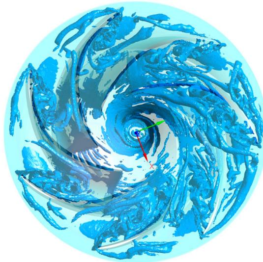
Figure 6. Vortex structures at 50%Pn (10% characteristic scale).
