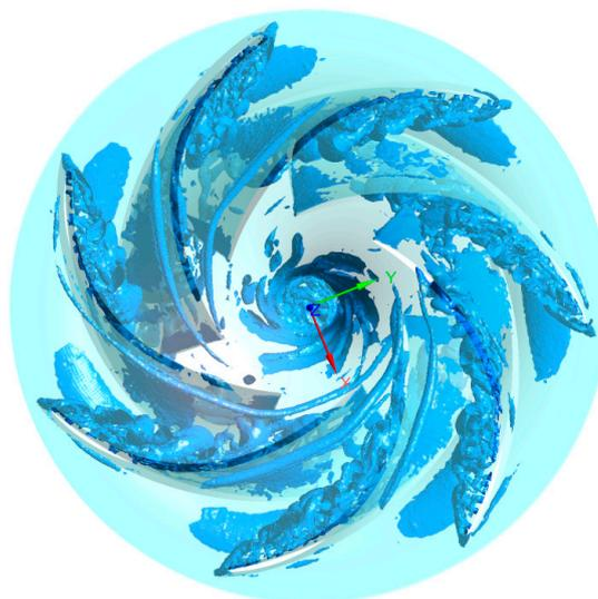
**Figure 4.** Vortex structures at 100%Pn (10% characteristic scale).
