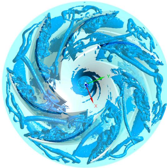
Figure 5. Vortex structures at 75%Pn (10% characteristic scale).
