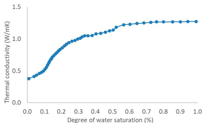
**Figure A1.** Thermal conductivity-Saturation curve for Bonny Silt.
