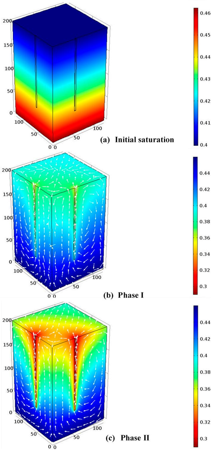
**Figure 5.** Saturation distribution: (a) before applying heat ( $t = 0$  days); (b) after applying heat in phase I ( $t = 4$  days) and (c) after applying heat in phase (II) ( $t = 4$  days). Arrows in figure (b,c) show the gas phase velocity field.
