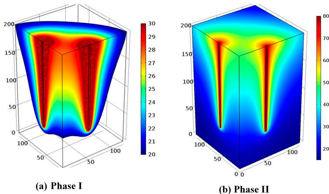
**Figure 4.** Temperature ( $^{\circ}\text{C}$ ) distribution in the domain after 4 days for (a) remediation phase and (b) storage phase. For the remediation phase, the part of the domain that has a temperature between 20–30  $^{\circ}\text{C}$  is shown. Only a quarter of the domain is presented.
