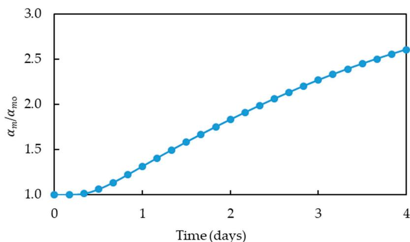
**Figure 6.** Ratio of carbon dioxide production after applying heat with respect to the reference value of carbon production at initial temperature ( $\alpha_m/\alpha_{mo}$ ) at a single point located in the middle of the domain.
