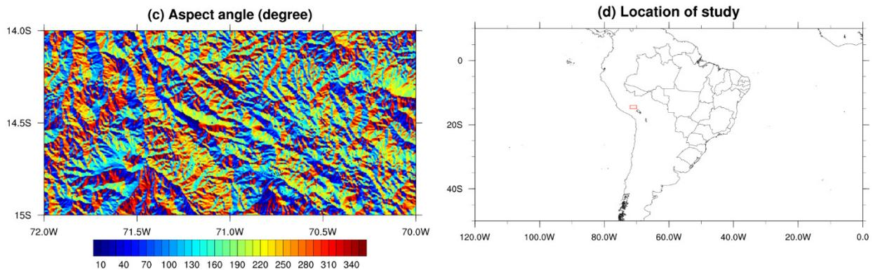
**Figure 1.** Topographic data produced from the digital elevation model (DEM) of the Shuttle Radar Topography Mission, part of Andes Mountains ( $72^{\circ}$  W: $70^{\circ}$  W,  $15^{\circ}$  S: $14^{\circ}$  S), (a) DEM (m), (b) slope height angle  $h_m$  (degree), (c) slope aspect angle  $a_m$  (degree), and (d) location of study indicated in red box.
