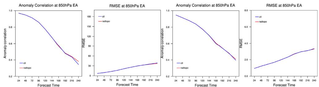
**Figure 7.** Time series of the anomaly correlation coefficient and RMSE (w.r.t ERA5) of geopotential height and temperature over Asia ( $60^{\circ}$  E: $144^{\circ}$  E,  $25.5^{\circ}$  N: $64.5^{\circ}$  N) at 850 hPa.
