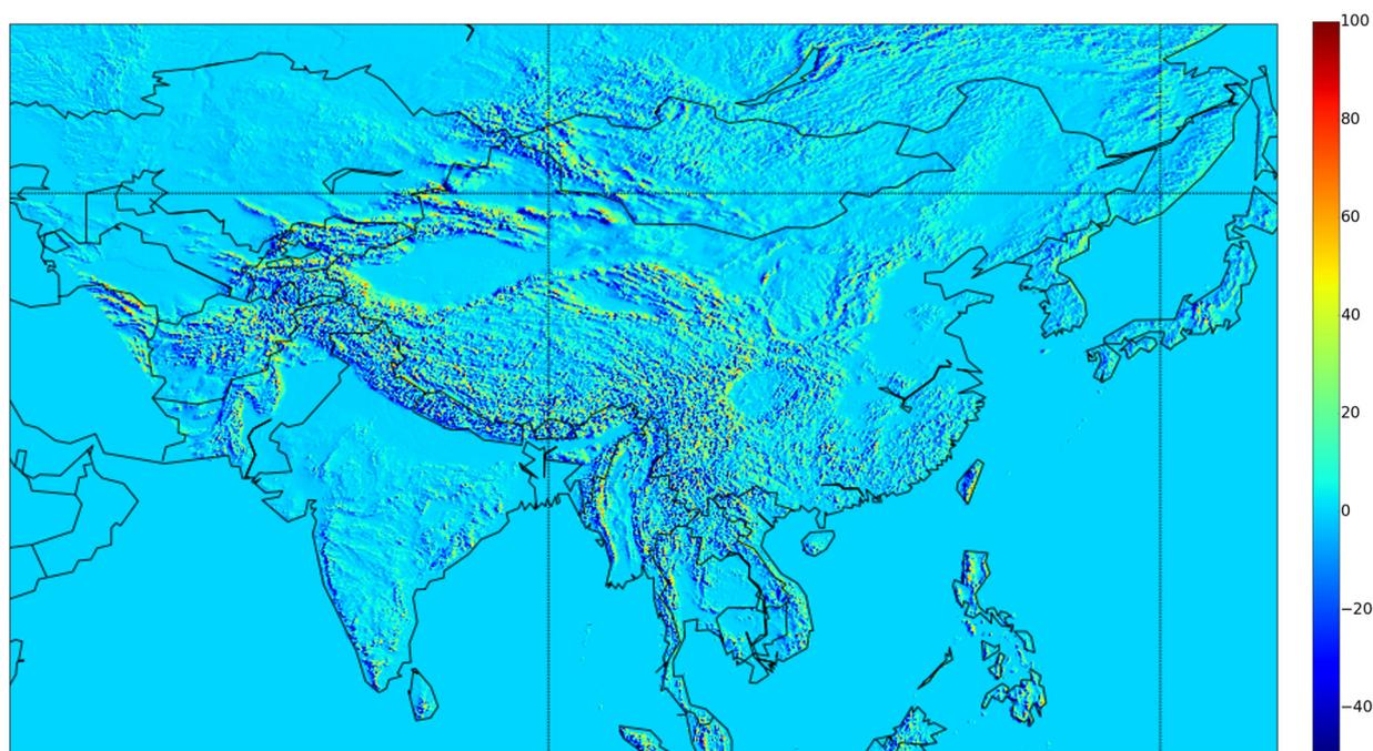
**Figure 4.** Flux difference [experiment (EXP) – control (CTL)] of the incident direct radiation at surface assuming no absorption and scattering ( $\text{Wm}^{-2}$ ) in offline simulation. North is at top, South at the bottom, West to the left, and East to the right. One grid size corresponds to 4500 km.
