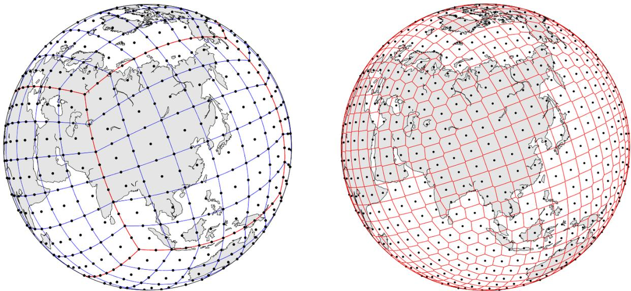
**Figure 2.** (left) Cubed sphere grid of Korean Integrated Model (KIM) and (right) Voronoi tessellation.
