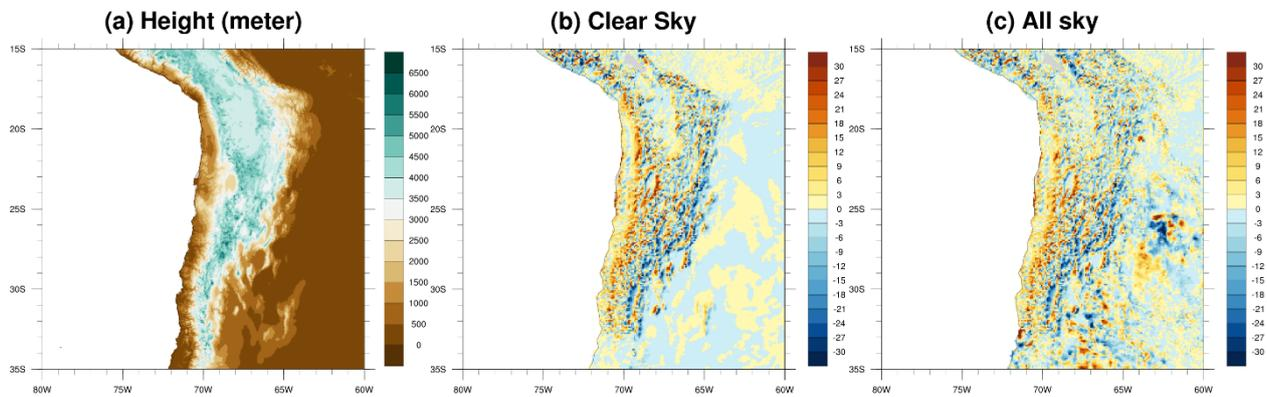
**Figure 5.** Flux difference [experiment (EXP) – control (CTL)] of the incident radiation at surface. The map shows the Andes Mountain area (80° W:60° W, 35° S:15° S). The flux is time averaged from 18 to 24 forecast hours (6 h frequency output). (a). Height(meter); (b) Clear Sky; (c) All sky.
