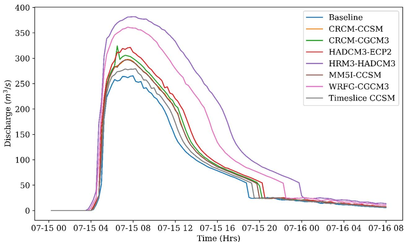
**Figure 5.** Discharge hydrograph for 6 h—100 years return period storm for different climate model.
