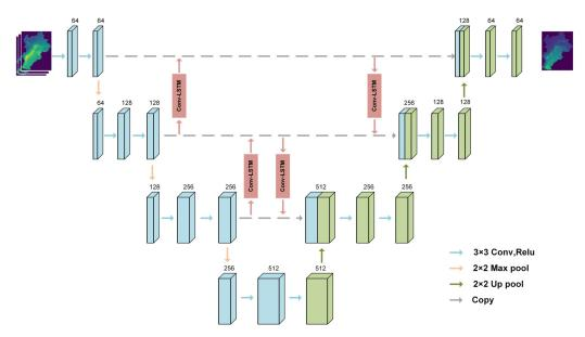
Figure 5. Structure of the U-convlstm model.
