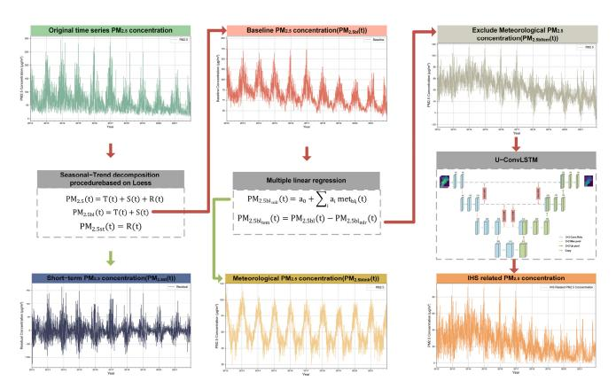
**Figure 4.** Process of meteorological and anthropogenic influence removal for estimating IHS impact on PM<sub>2.5</sub> concentrations (illustrated using a single pix value).
