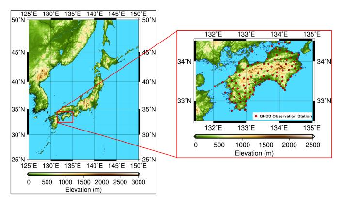
**Figure 1.** Locations of the target region, along with GNSS observation stations. The base map shows the elevation, which was mapped using ASTER GDEM data. The red dots indicate the locations of the GNSS observation stations.
