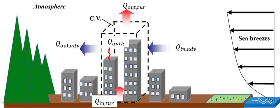
Figure 1. Concept of the heat balance mechanism in an urban space [1,18].
