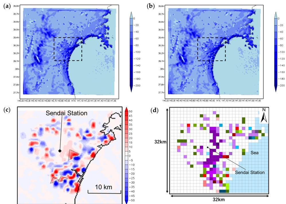
**Figure 10.** Distributions of the advection component of sensible heat balance [MW] in the daytime. (a) In Case lu\_2002; (b) in Case lu\_2022; (c) changes in the advection component of sensible heat balance (between Case lu\_2022 and Case lu\_2002); and (d) land use changes between 2002 and 2022 in Sendai (reposted Figure 4).
