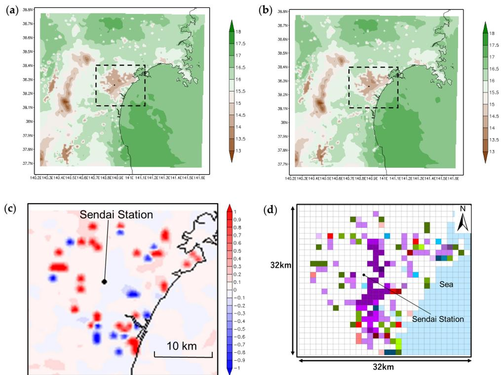
**Figure 9.** Daytime specific humidity [g/kg'] distributions. (a) In Case lu\_2002; (b) in Case lu\_2022; (c) specific humidity differences (between Case lu\_2022 and Case lu\_2002); and (d) land use changes between 2002 and 2022 in Sendai (reposted Figure 4).
