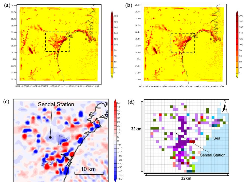
**Figure 11.** Distributions of the advection component of latent heat balance [MW] in the daytime. (a) In Case lu\_2002; (b) in Case lu\_2022; (c) changes in the advection component of latent heat balance (between Case lu\_2022 and Case lu\_2002); and (d) land use changes between 2002 and 2022 in Sendai (reposted Figure 4).
