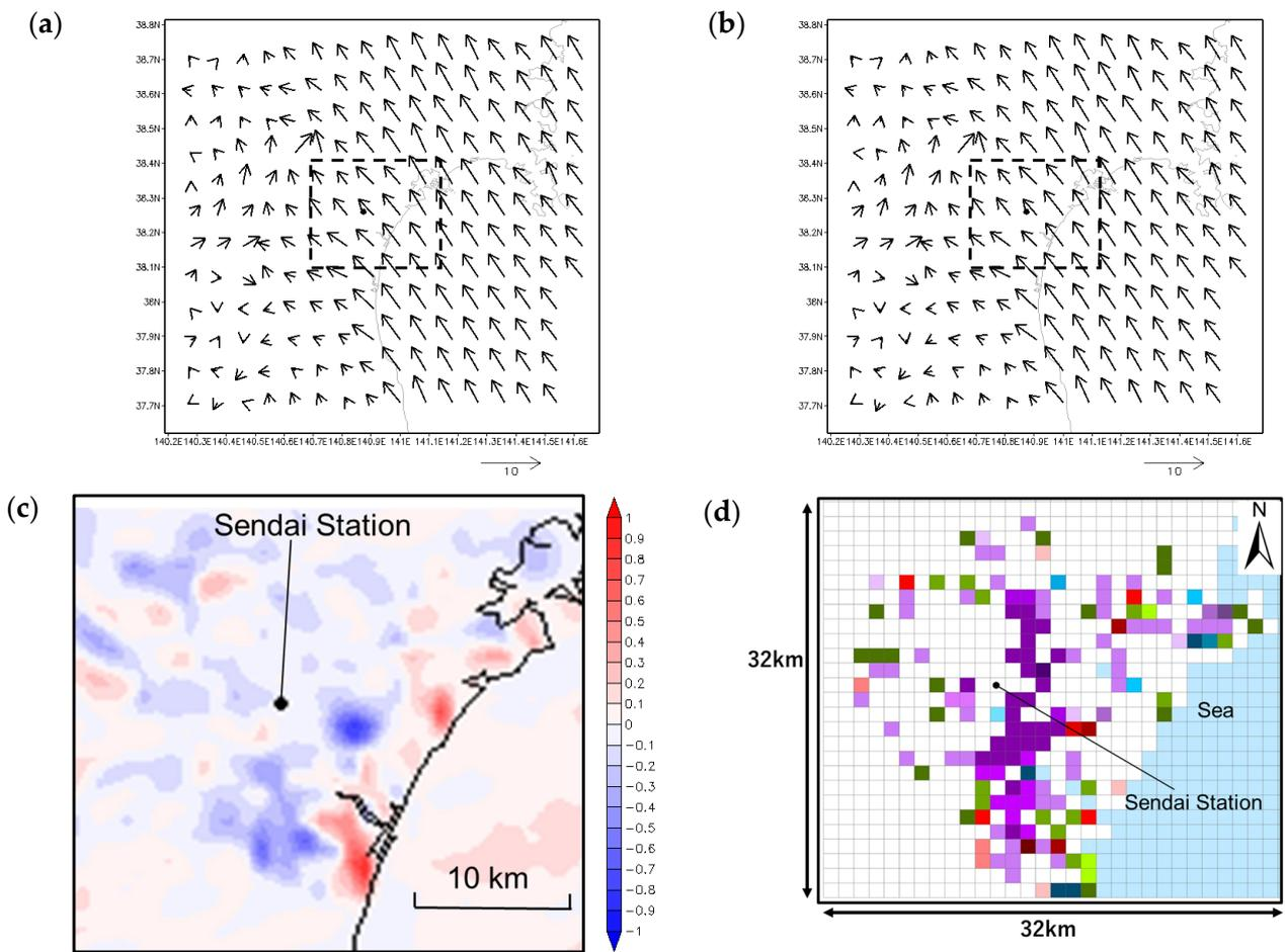
**Figure 7.** Daytime wind {m/s} fields. (a) In Case lu\_2002; (b) in Case lu\_2022; (c) scalar difference of wind speed (between Case lu\_2022 and Case lu\_2002); and (d) land use changes between 2002 and 2022 in Sendai (reposted Figure 4).
