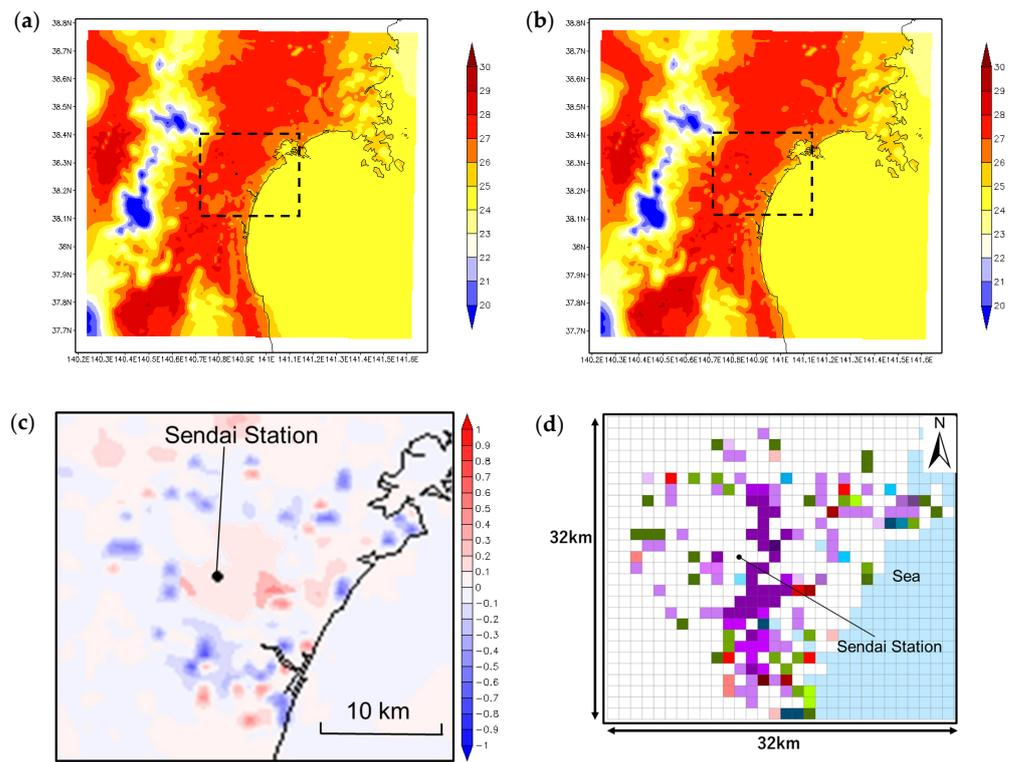
**Figure 8.** Daytime air temperature [°C] distributions. (a) In Case lu\_2002; (b) in Case lu\_2022; (c) air temperature differences (between Case lu\_2022 and Case lu\_2002); and (d) land use changes between 2002 and 2022 in Sendai (reposted Figure 4).
