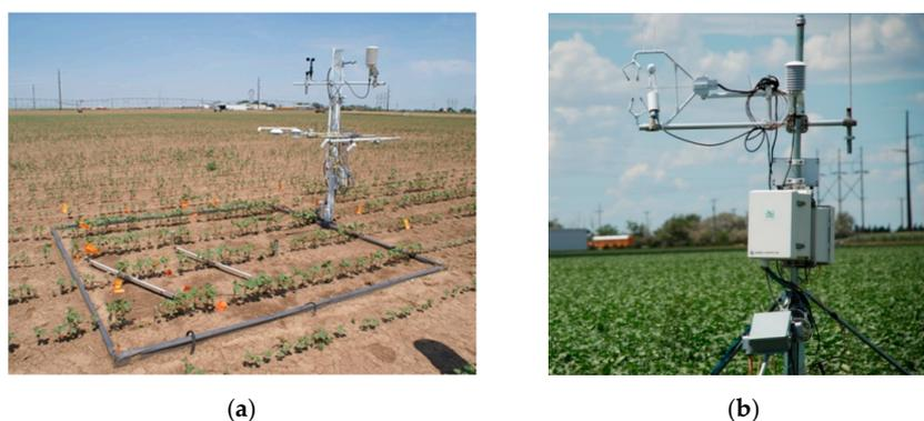
**Figure 1.** (a) Lysimeter box with micrometeorological instrumentation and (b) eddy covariance system. Photographs courtesy of Dr. José Luis Chávez.
