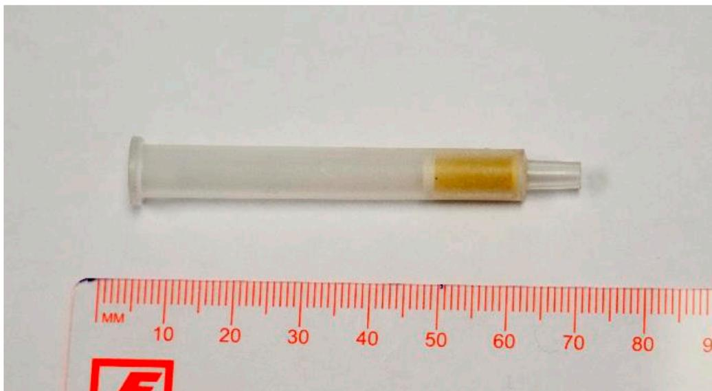
**Figure S1.** Image of Cl<sub>2</sub>-RPGE tube, next to a ruler for size measurement.
