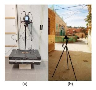
Figure 3. Instruments used for the study fields: (a) meteorological station, (b) fish-eye camera.
