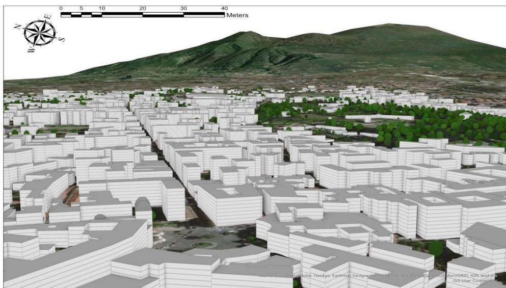
**Figure 4.** 3D Urban Model of the city of Portici including buildings and vegetation derived by geographical information systems (GIS) and LiDAR data. View of the Park of the Reggia and the main square—Piazza San Ciro.
