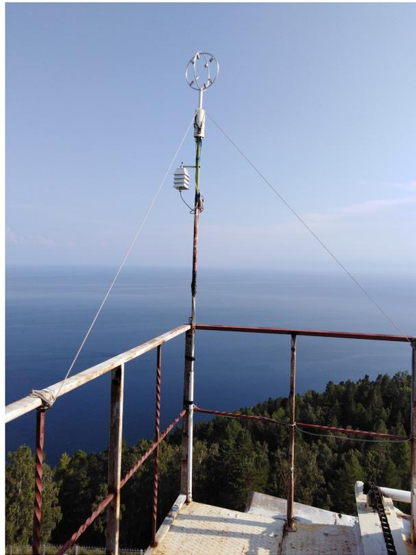
**Figure 1.** Meteorological sensor mounted on the mast, large solar vacuum telescope.
