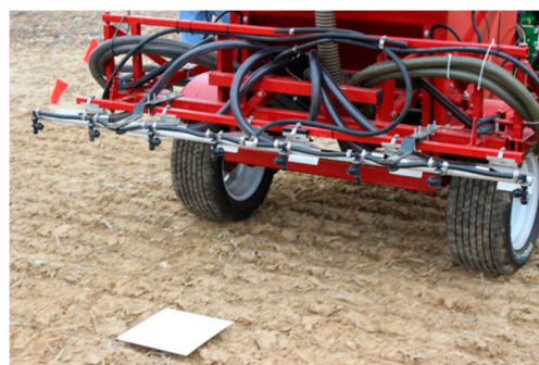
Figure 5. Broadcast seeding with a Valmar 1255 Twin Rotor air seeder.
