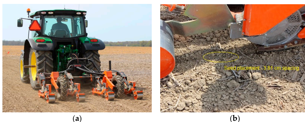
Figure 6. Direct seeding: (a) Stanhay air drill seeder; (b) Seed in row at 3.81 cm spacing.
