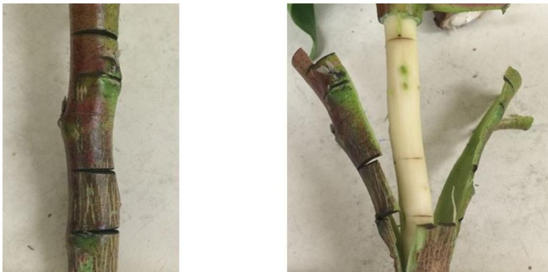
**Figure 20.** Figures details the results shown from laser power tests that were performed on freshly harvested field-grown cotton plants to determine cutting depth versus laser-power. The figure on left shows the stalk as it was immediately after laser cutting. The figure on right is after removal of the bark to reveal the depth of the laser cut. To ensure complete phloem termination, the white wood should show a laser scar all the way around the perimeter.
