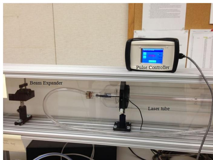
**Figure 4.** Experimental micro-controller-based computer-numerical-controlled (CNC) CO<sub>2</sub> laser treatment system designed to provide precise control over the laser treatment time and energy density.
