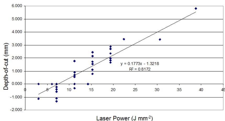
**Figure 21.** Figure details the regression analysis for the laser power tests that were performed on freshly harvested field-grown cotton plants to determine cutting depth versus laser-power. Results are from plants ranging in height from 250 mm to 725 mm. A zero depth corresponds to the depth where the laser just penetrated through the bark and the phloem tissue. The negative depth indicates insufficient power.
