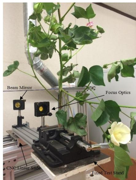
**Figure 5.** Experimental micro-controller based CNC CO<sub>2</sub> laser treatment system designed to provide precise control over the laser treatment time and energy density.
