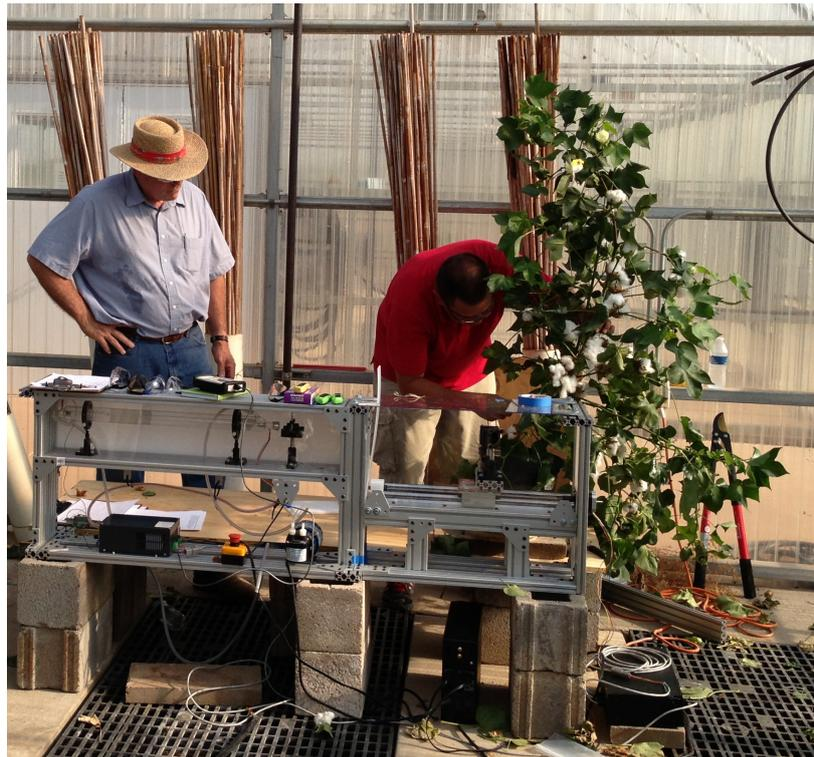
**Figure 7.** Girdling with CNC CO<sub>2</sub> laser treatment system on greenhouse-grown cotton plants.
