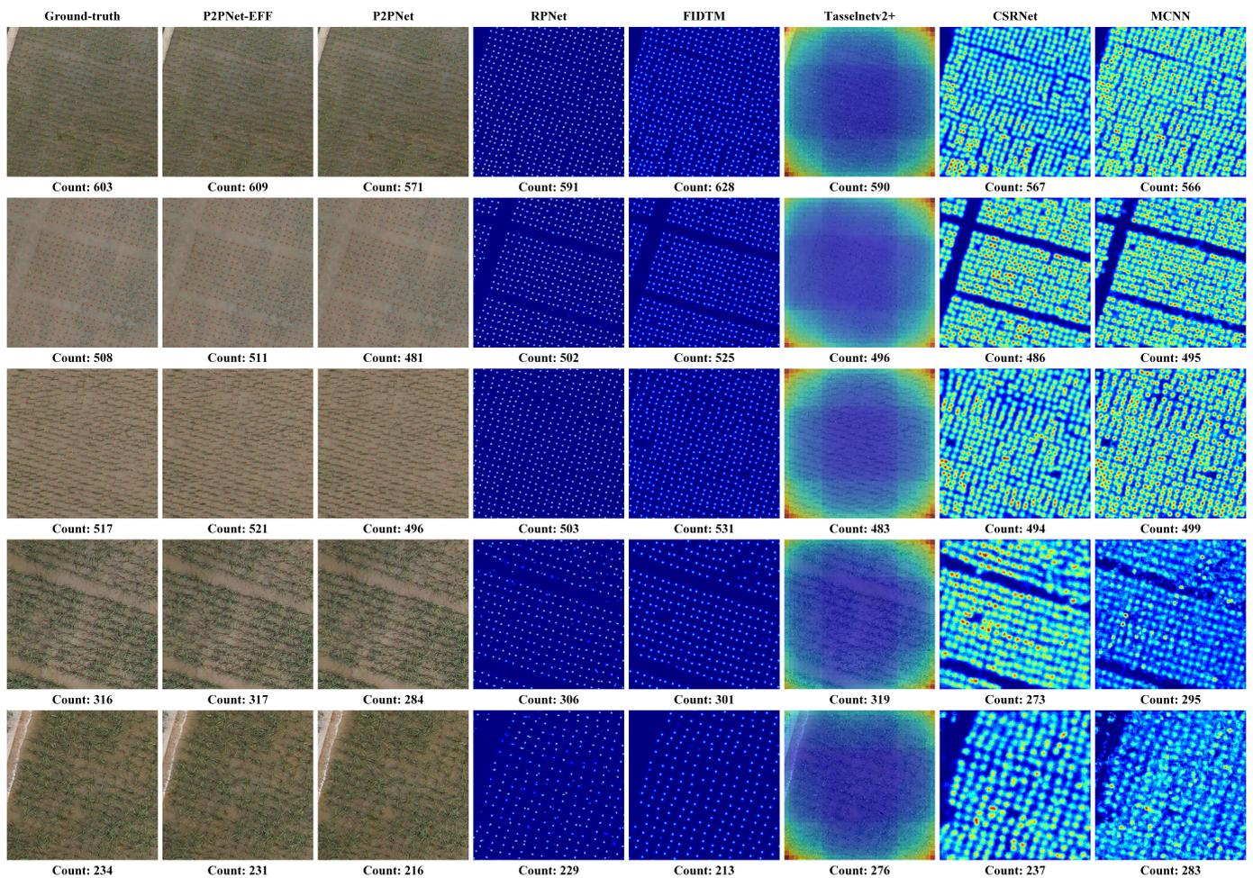
**Figure 6.** Visualization of the results obtained by the various methods on the URCAL dataset. In the ground truth, “count” denotes the number of ground-truth points, while in the other methods, “count” signifies the counts predicted by each respective method.
