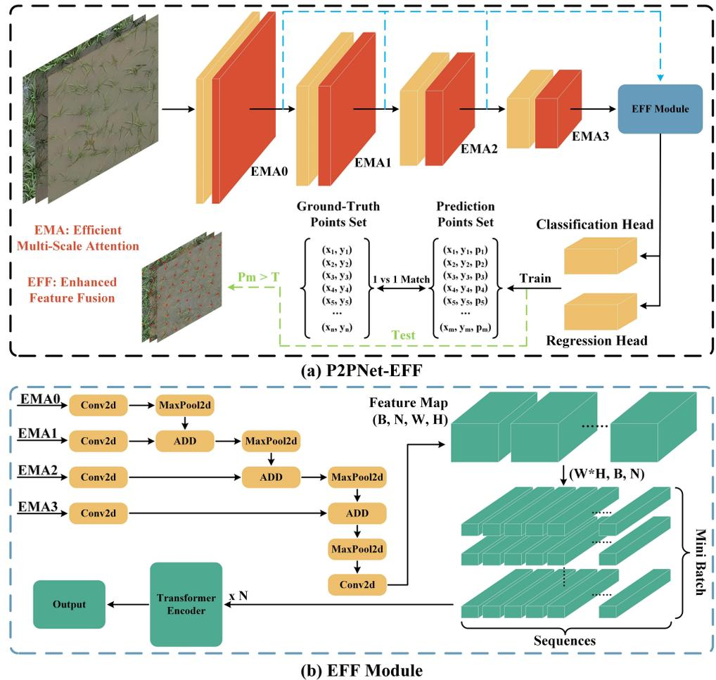
**Figure 4.** (a) Overall architecture of P2PNet-EFF, where  $(x, y)$  are point coordinates and  $p$  is the prediction confidence generated by the classification header.  $T$  in  $P_m > T$  is the threshold for filtering labels during model inference. (b) Detailed flowchart of EFF, where  $(B, N, W, H)$  denotes the shape of the feature map,  $B$  is the batch size,  $N$  is the number of channels, and  $W, H$  are the width and height, respectively.
