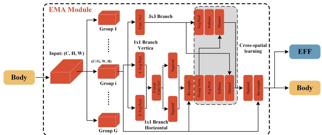
Figure 5. The structure of efficient multi-scale attention module.
