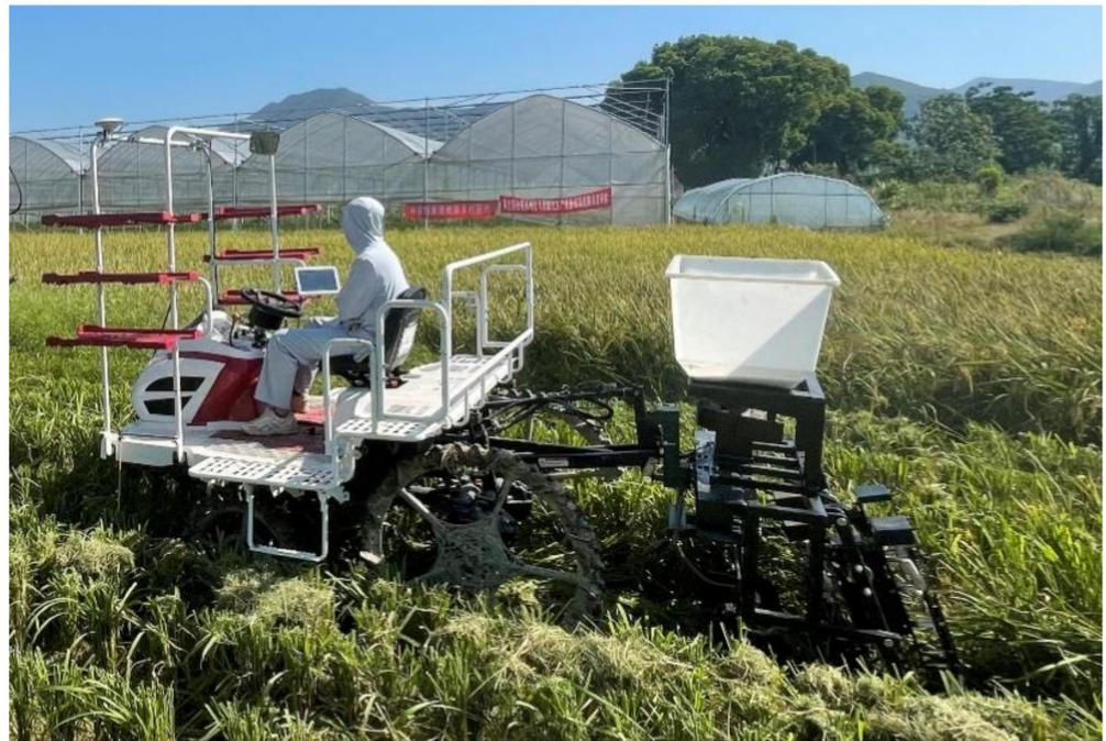
**Figure 1.** The righting machine for crushed stubble after mechanical harvest.
