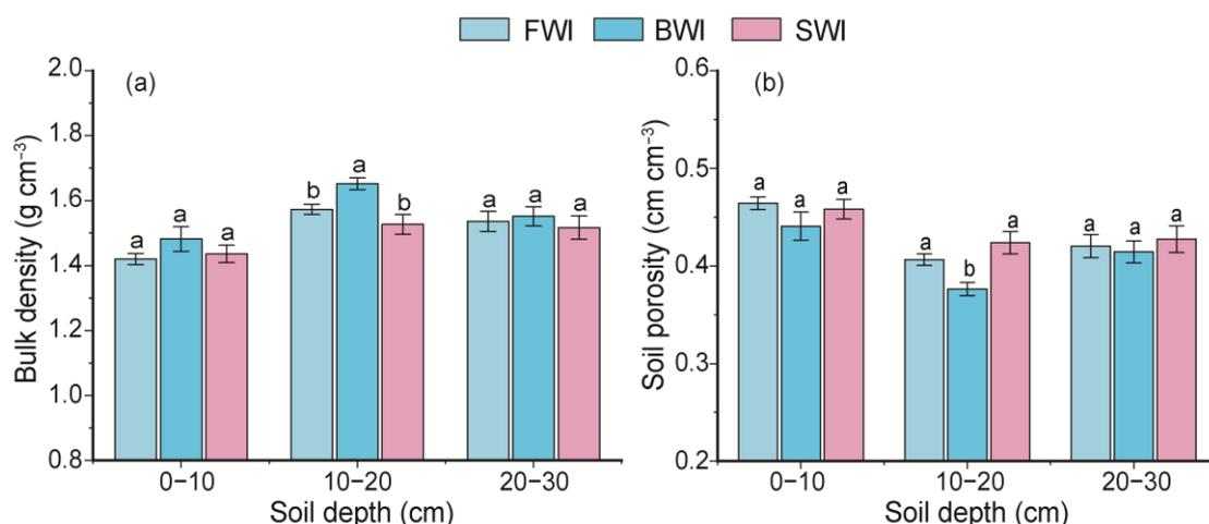
**Figure 2.** Comparison of bulk density (a) and porosity (b) in different layers (0–10 cm, 10–20 cm, and 20–30 cm) between the fresh (FWI), brackish (BWI), and salt (SWI) water irrigation treatments. Error bars represent standard errors. The different lower-case letters indicate significant differences between treatments ( $p < 0.05$ ; Fisher's LSD test).
