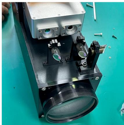
**Figure 3.** A handheld Raman Spectroscopy detection device.
