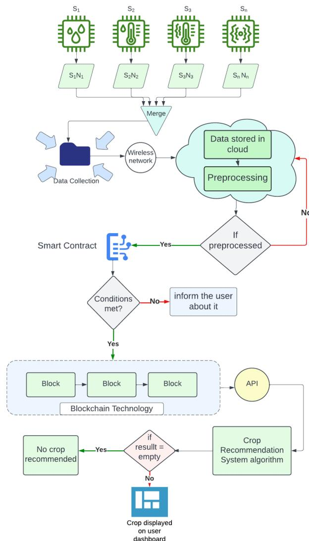
**Figure 2.** Work flow of the crop recommendation system.
