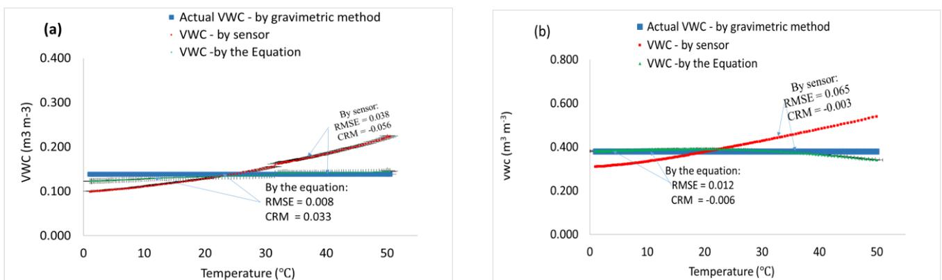
**Figure 11.** Comparison between VWC values measured by sensor, by gravimetric method, and by proposed L&O correction equation with gradual increase in soil temperature at  $2.42 dS m^{-1}$  at (a) field capacity moisture and (b) saturated points.
