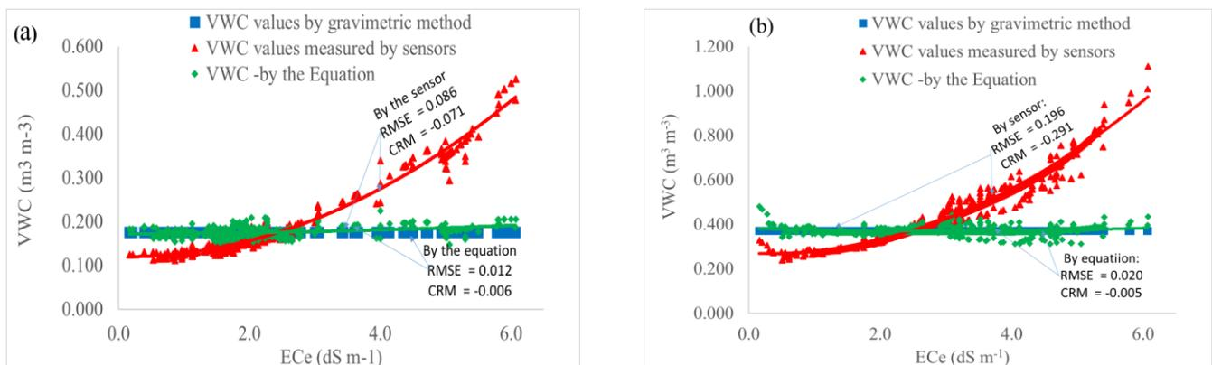
**Figure 10.** Comparison between VWC values measured by sensor, by gravimetric method, and by proposed L&O correction equation with a gradual increase in soil EC at  $25 \text{ }^\circ\text{C}$ , tested at (a) soil moisture at field capacity and (b) soil moisture at saturated point.
