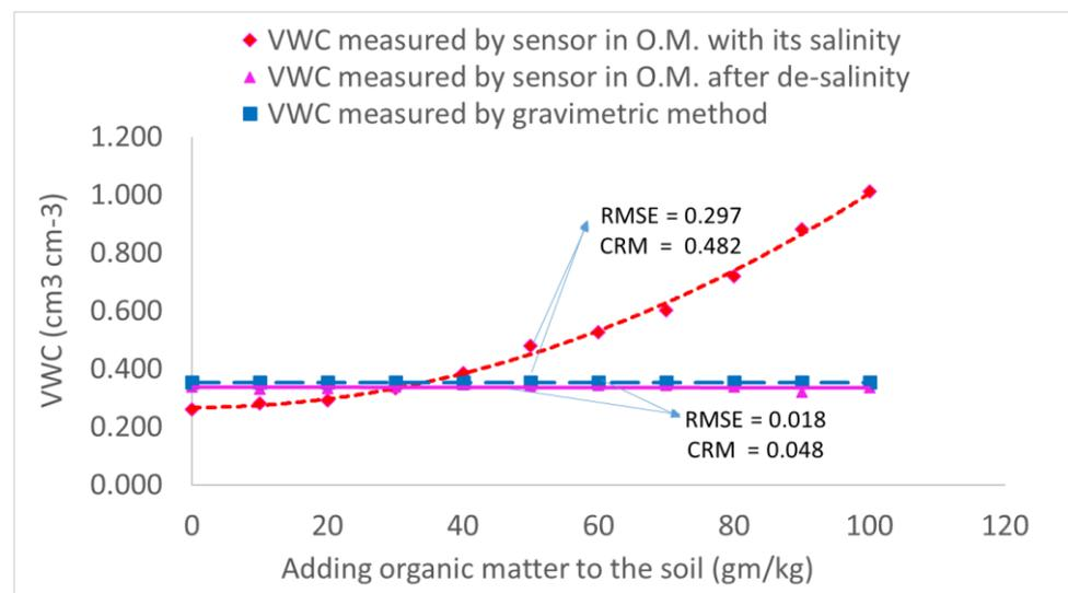
**Figure 6.** Influence of organic matter on sensor measurements before and after desalination.
