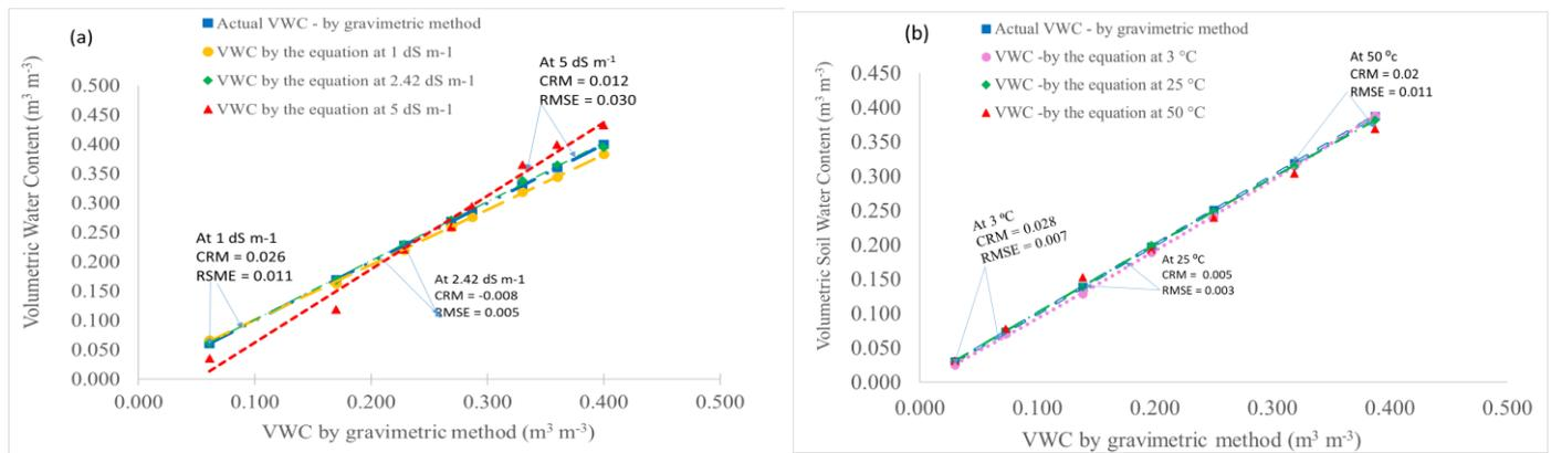
**Figure 9.** Comparison between actual VWC values measured by gravimetric method and calculated by L&O equation in graded increasing soil moisture at three levels of (a) EC and (b) temperature.
