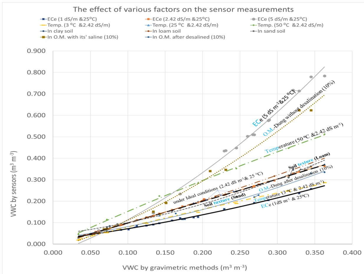
Figure 2. The influence of various factors on sensor measurements.
