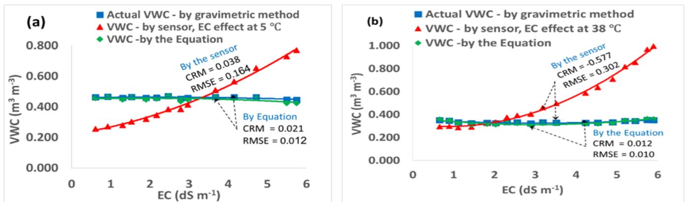
Figure 12. Comparison between VWC values measured by sensors using gravimetric method and proposed L&O correction equation with gradual increase in soil salinity at (a) 5 °C and (b) 38 °C.
