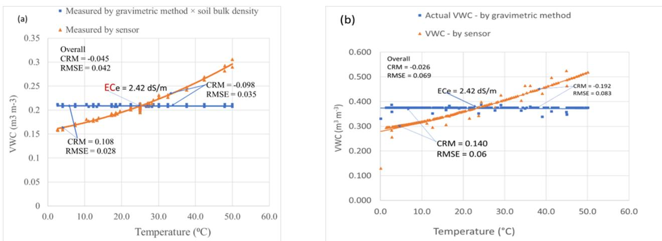
**Figure 5.** Influence of soil temperature on sensor measurements at (a) field capacity and (b) saturated points.
