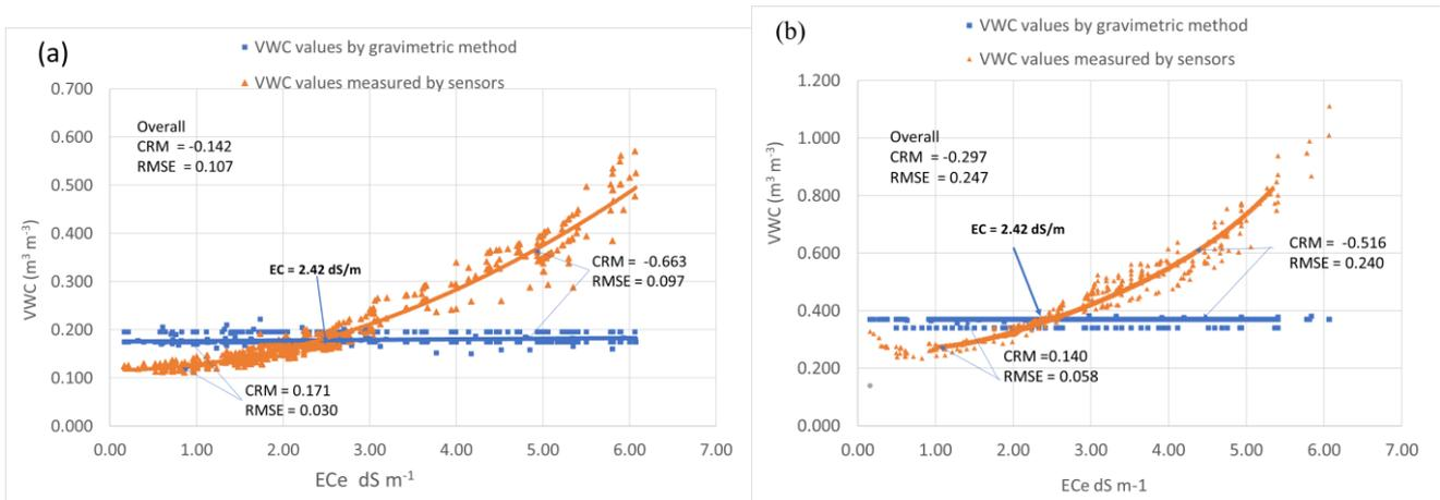
**Figure 4.** Influence of EC on sensor measurements at (a) field capacity and (b) saturated points.
