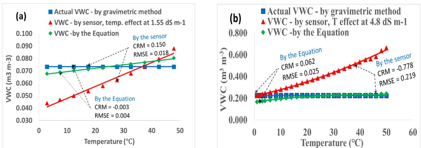
Figure 13. Comparison between VWC values measured by the sensors using gravimetric method and calculated by proposed L&O correction equation with gradually increasing soil temperature at (a) 1.55 dS m<sup>-1</sup> in low moisture and (b) 4.62 dS m<sup>-1</sup> in field-capacity moisture.
