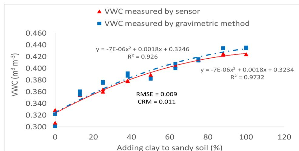
**Figure 7.** Influence of soil texture on sensor measurements.
