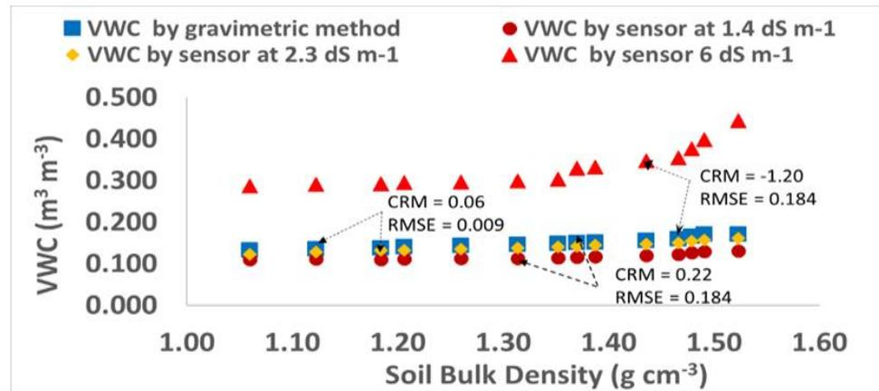
**Figure 8.** Influence of soil bulk density on sensor measurements in low-salinity (1.4 dS m<sup>-1</sup>), moderate (2.3 dS m<sup>-1</sup>), and high-salinity soil (6 dS m<sup>-1</sup>).
