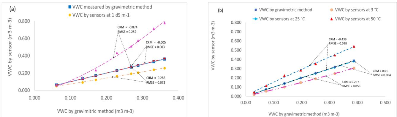
Figure 3. Correlation between actual VWC by gravimetric method and the sensor at three levels of (a) salinity concentration and (b) temperature.
