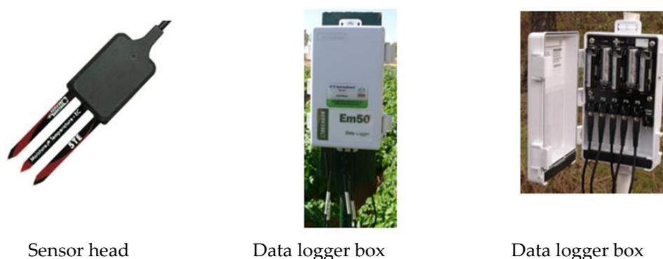
**Figure 1.** ECH2O-5TE sensors in all rubs of testing.
