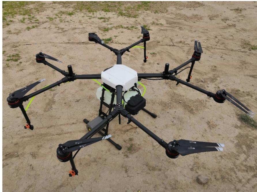
**Figure 1.** DJI AGRAS MG-1P UASS applied in spray drift tests.
