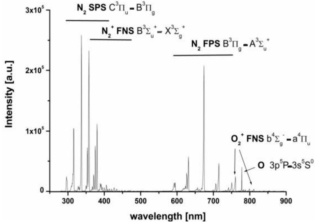
Figure 3. Emission spectrum indicating some of the radiative reactive species produced.
