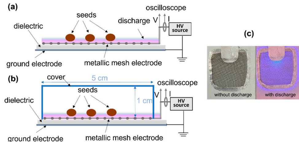
**Figure 1.** Schematic representation of the flexible configuration used for the seed treatments: (a) direct plasma, (b) with cover, (c) picture of the electrode from above without and with discharge.
