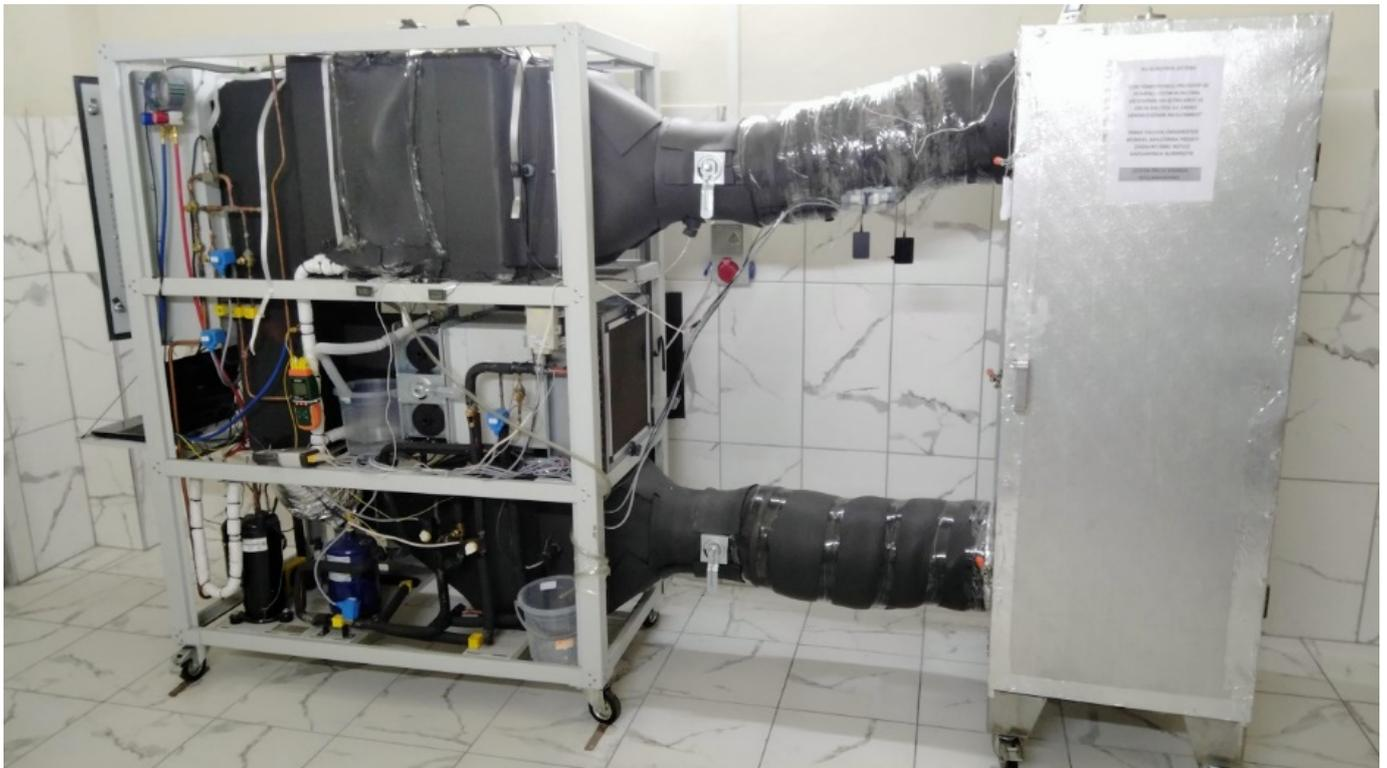
**Figure 3.** The closed circuit HPD system specially designed for this study.
