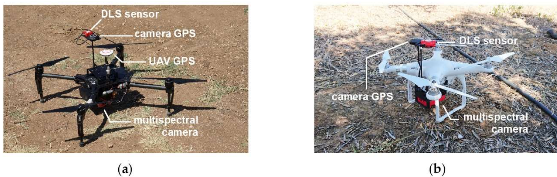
Figure 2. Aerial image acquisition equipment: (a) DJI Matrice 100-based setup; (b) DJI Phantom 3 Advance-based setup.
