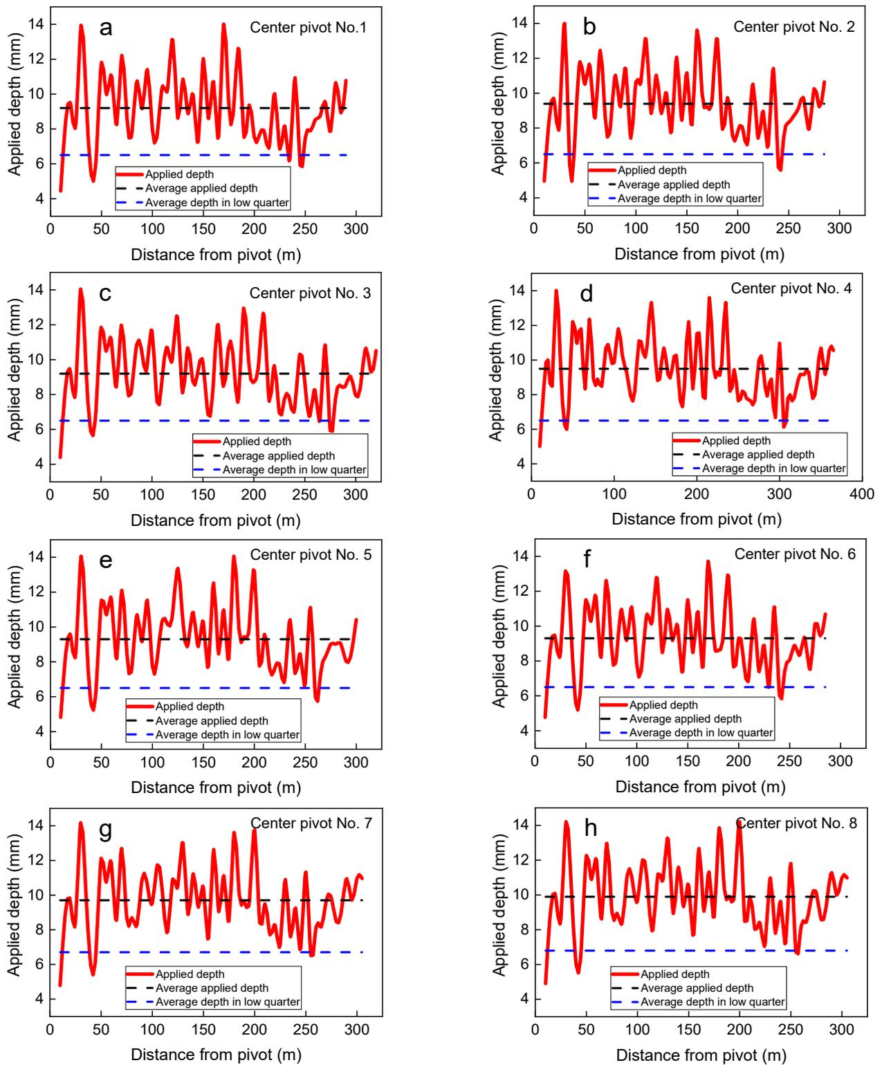
**Figure 6.** Water distribution patterns with the average depths and the average low quarter depths of application measured from the tested center pivot irrigation systems with standard laterals. The symbols (a–h) correspond to the tested center pivot systems numbered 1 to 8.
