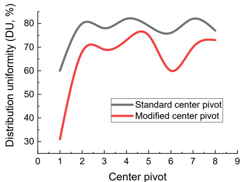
**Figure 9.** A comparison between the distribution uniformity (DU) for both the standard- and modified-laterals of the tested center pivot irrigation systems.
