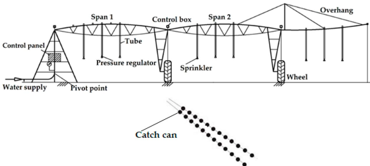
Figure 5. Catch cans arrangement for the performance evaluation of the center pivot irrigation systems.
