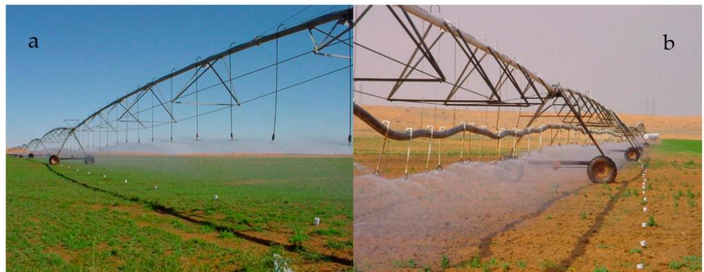
Figure 3. Two types of center pivot irrigation systems employed in the study regions with standard lateral (a) and modified lateral (b).
