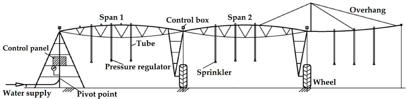
Figure 4. Schematic of the center pivot irrigation system.
