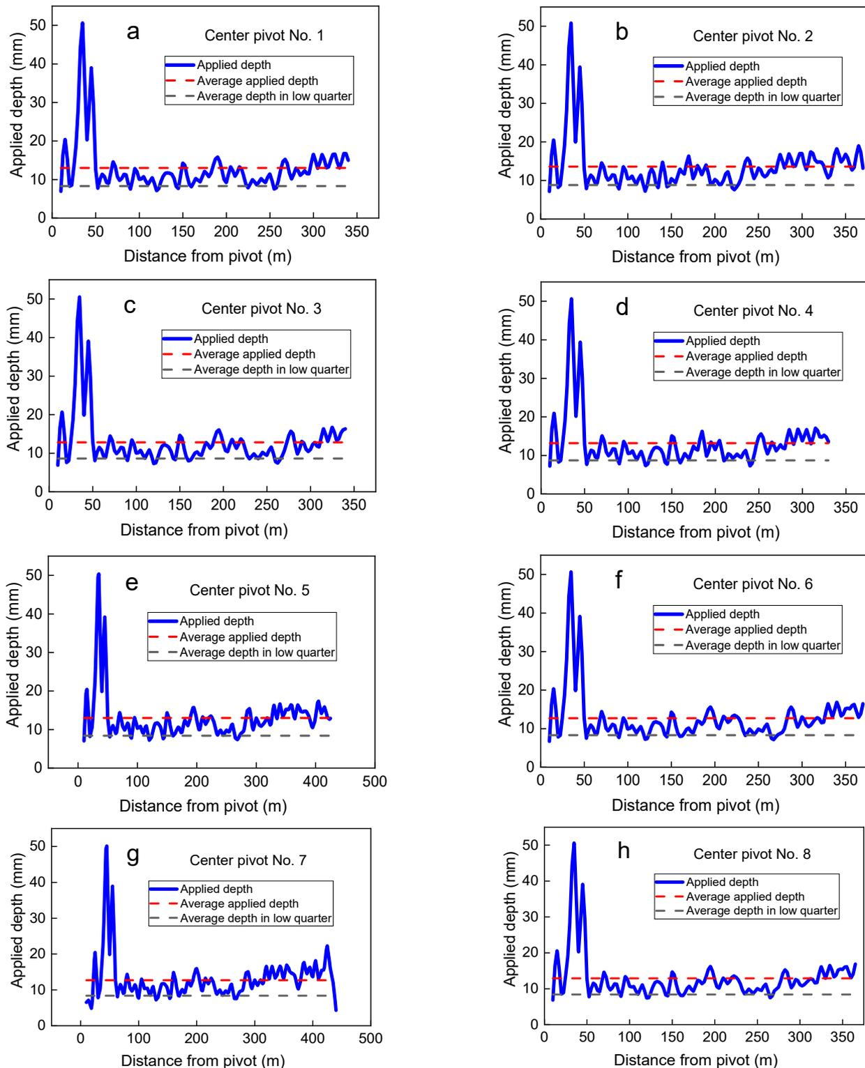
**Figure 7.** Water distribution patterns with the average depths and the average low quarter depths of application measured from the tested center pivot irrigation systems with modified laterals. The symbols (a–h) correspond to the tested center pivot systems numbered 1 to 8.
