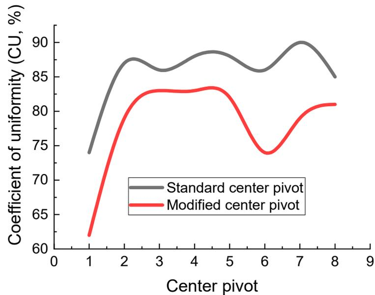
**Figure 8.** A comparison between the coefficient of uniformity (CU) for both the standard- and modified-laterals of the tested center pivot irrigation systems.
