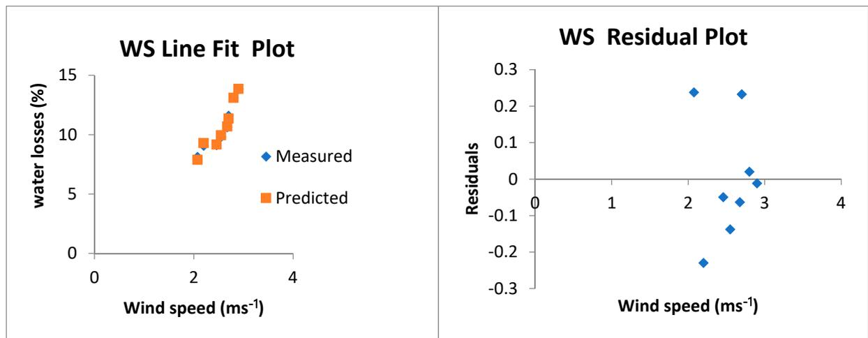
Figure 10. Measured and predicted water losses of the MLR model using the wind speed (WS) dataset.
