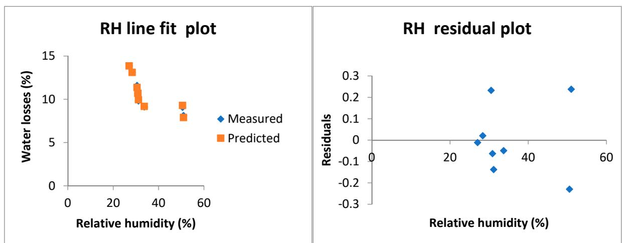
Figure 12. Measured and predicted water losses of the MLR model using the relative humidity (RH) dataset.
