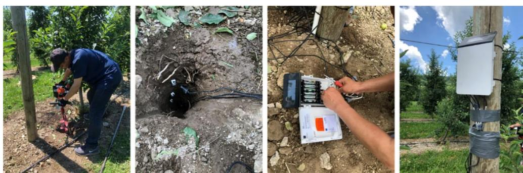
**Figure 3.** Soil moisture sensor systems setup in the orchard. From left to right: drill a hole for sensors, install sensors at different depths, connect sensors to a datalogger, place the datalogger to a pole.
