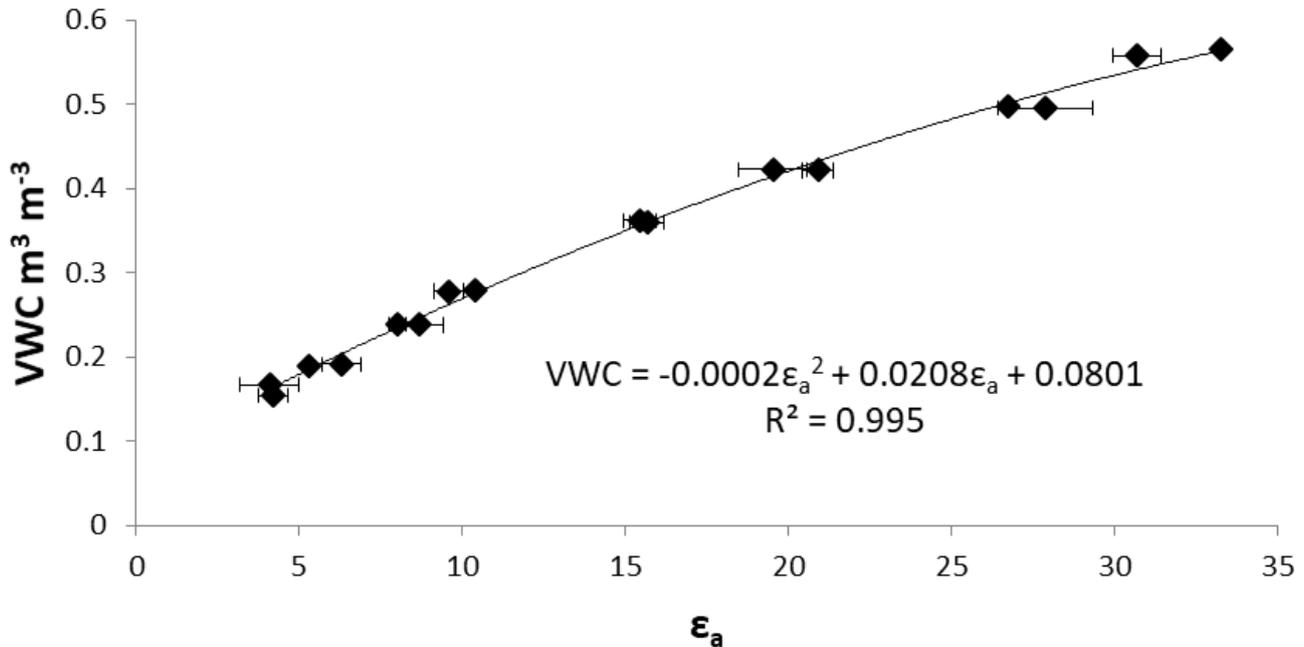
**Figure 1.** Relationship between volumetric water content (VWC) of a peat:perlite (3:1 *v:v*) mixture and the dielectric output ( $\epsilon_a$ ) of GS3 sensors. Each point is the average of two readings from two different sensors at a specific substrate VWC level. Horizontal bars represent  $\pm$  ES of the average value.
