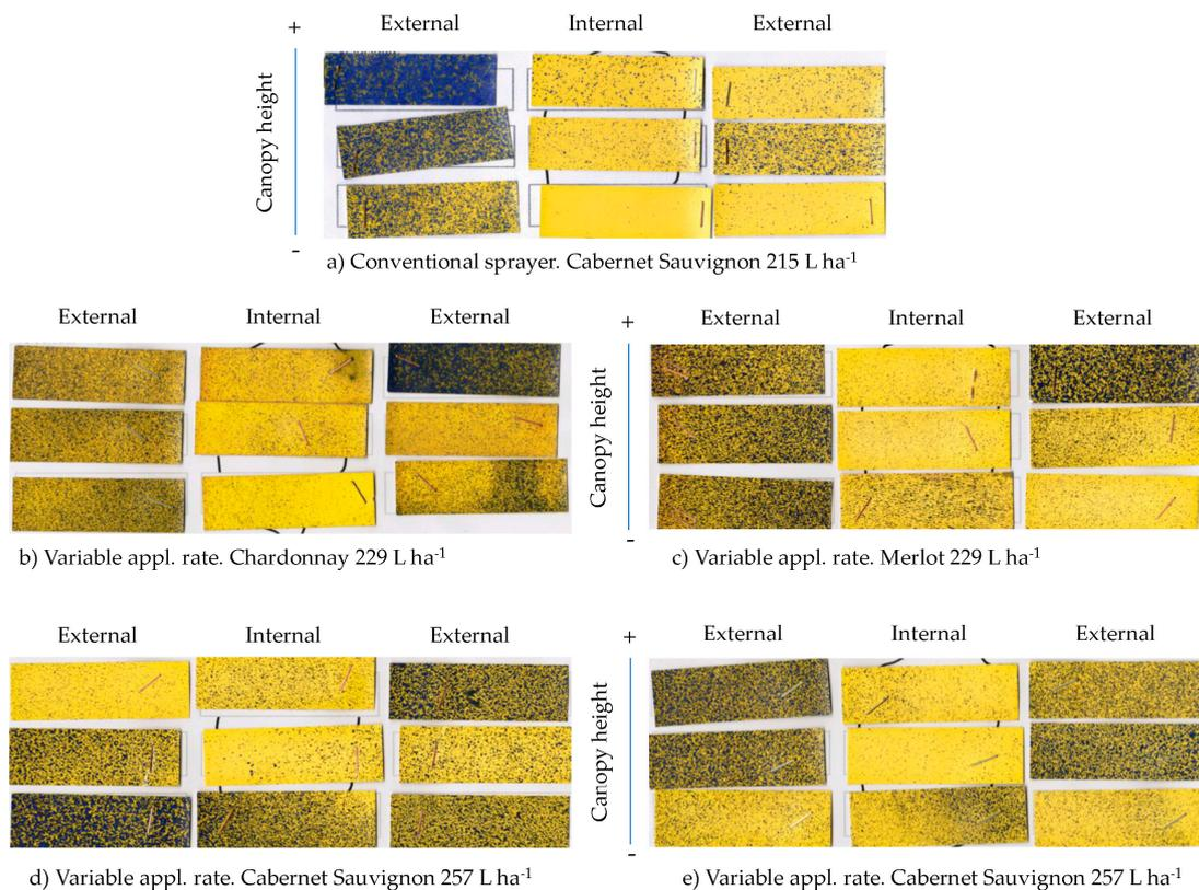
**Figure 10.** Coverage (WSP) obtained with conventional spray application (CONV) (a), in comparison with coverage obtained at the four selected varieties when using variable rate application (VRA) (b–e).
