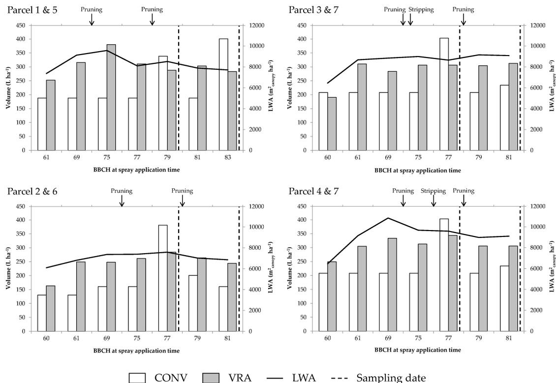
**Figure 11.** Volume rate applied in conventional and variable rate parcels in each spray application. Time of the evaluation of the biological efficacy (sampling time) as well as pruning and stripping task are marked.
