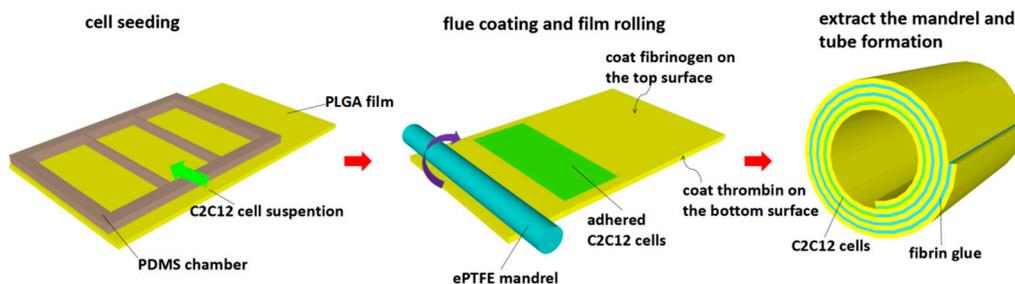
**Figure S7.** Fabrication scaffolds with one layer of cells seeded (illustrating the cell distribution for cell adhesion, proliferation and migration tests by SEM). The only difference from the fabrication of the scaffolds with three layers is that only the middle part of the chamber is seeded with cell suspension.
