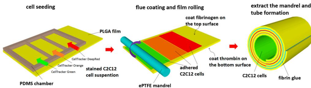
**Figure S6.** Fabrication scaffolds with stained cells (illustrating the cell distribution for cell migration test by a fluorescent assay). The only difference from the fabrication process for scaffolds without cells is that cells were stained by different dyes before seeding (The cells on the first, second, and third layer were stained with CellTracker Green, CellTracker Orange, and CellTracker DeepRed, respectively).
