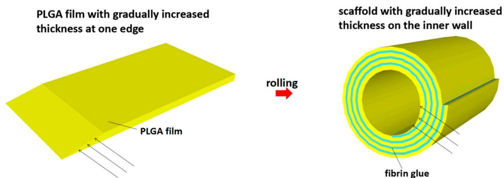
**Figure S14.** A possible design for the solution to the internal edge of the rolling-based scaffolds. A PLGA film with gradually increased thickness at its edge (arrow heads) might be helpful.
