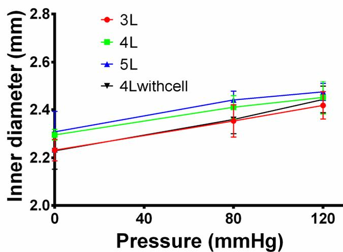
Figure S11. The pressure-inner diameter curve of the scaffolds.
