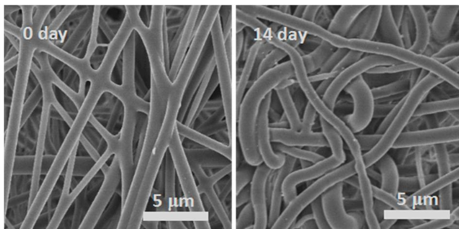
**Figure S8.** The morphology of PLGA fibers before and after 14 days' degradation in DMEM at 37°C with 5% CO<sub>2</sub>.
