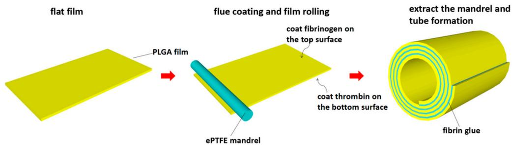
**Figure S2.** Fabrication scaffolds without cells. The PLGA films were cut into rectangles with proper
