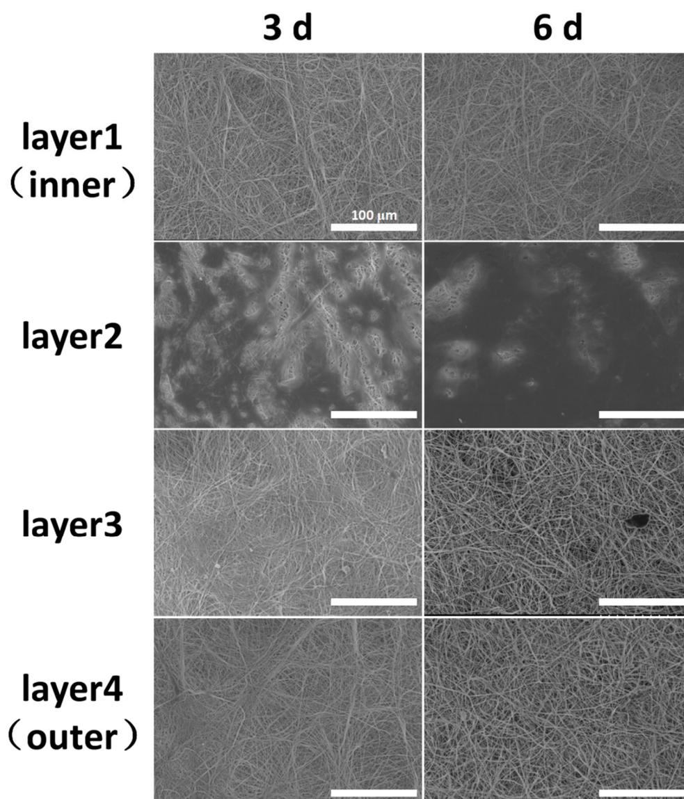
**Figure S13.** SEM images of and cell proliferation and cell migration after 3 d and 6 d in scaffolds. The second layer is the cell seeded layer. Cell proliferation can be observed different time points from the second layer. Cell migration between layers can be observed from inner to outer layers of the scaffolds.
