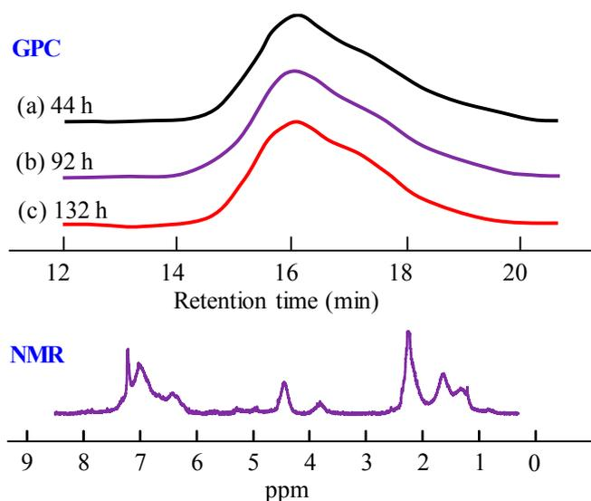
**Figure 3.** GPC and NMR results of the extracted materials from the ETFE-g-poly(CMS) film.
