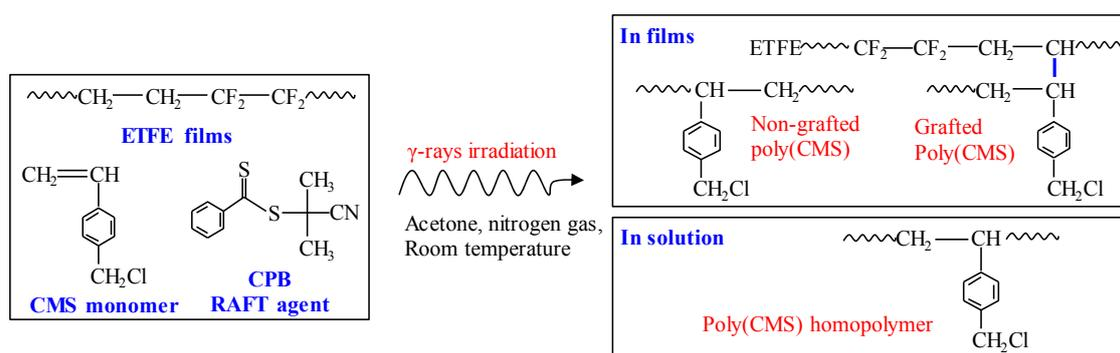
**Scheme 1.** Process for the simultaneous radiation grafting of chloromethylstyrene (CMS) onto ethylene-tetrafluoroethylene copolymer (ETFE) films.
