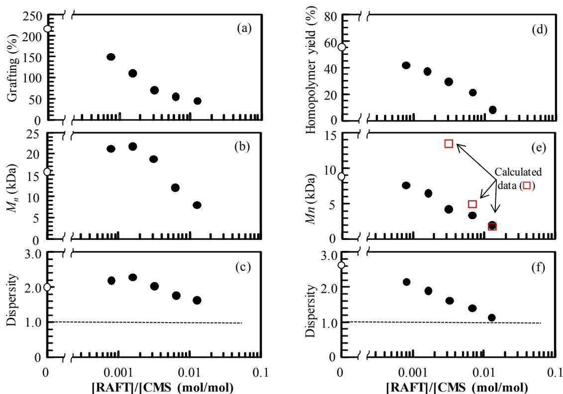
**Figure 6.** (a) Degree of grafting, (b)  $M_n$ , (c) dispersity of the extracted poly(CMS) from grafted ETFE films, and (d) homopolymer yield, (e)  $M_n$ , (f) dispersity of the homopolymer in the monomer solution as a function of the mole ratio of  $[\text{RAFT}]/[\text{CMS}]$ . Irradiation dose rate, 1.0 kGy/h; total irradiation dose, 50 kGy;  $[\text{RAFT}]/[\text{CMS}]$ , 0.014.
