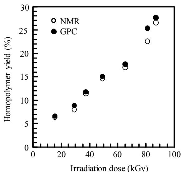
**Figure 2.** Homopolymer yield in the irradiated monomer solution determined by NMR and GPC methods as a function of the total irradiation dose. Dose rate, 1.0 kGy/h; [RAFT]/[CMS], 0.014; room temperature.
