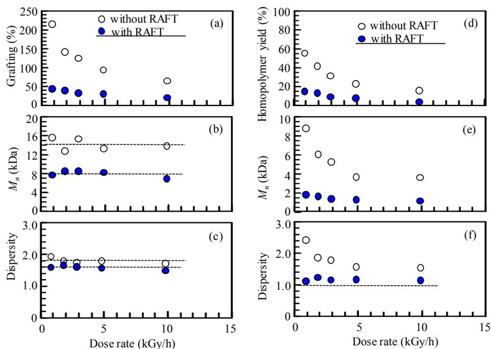
**Figure 5.** (a) Degree of grafting, (b)  $M_n$ , (c) dispersity of the extracted poly(CMS) in the ETFE films, and (d) homopolymer yield, (e)  $M_n$ , (f) dispersity of the homopolymer in the monomer solution as a function of the irradiation dose rate. Total irradiation dose, 50 kGy; [RAFT]/[CMS], 0.014.
