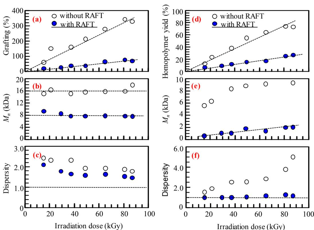
**Figure 4.** (a) Degree of grafting, (b) average molecular weight ( $M_n$ ), (c) dispersity of the extracted poly(CMS), and (d) homopolymer yield, (e)  $M_n$ , (f) dispersity of the homopolymer in monomer solution as a function of the irradiation dose. Irradiation dose rate, 1.0 kGy/h; [RAFT]/[CMS], 0.014.
