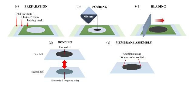
**Figure 1.** Phases of the preparation of the elastomeric electrode: (**a**) A pouring mask with a shaped cut is laid on the Elastosil<sup>®</sup> film; (**b**) A mixture of polydimethylsiloxane (PDMS), carbon black, and isopropanol is poured; (**c**) The excess material is removed by blading; (**d**) After crosslinking, two membranes are bonded; (**e**) The membrane is assembled.
