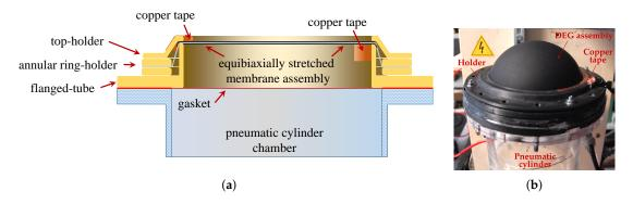
**Figure 2.** (a) Schematic of the membrane assembly (screws are not represented): the membrane assembly is secured on an annular ring holder and squeezed on a flanged-tube (that provides it with a certain pre-stretch), which is fixed to the ring-holder by means of a top holder. (b) A picture of the inflated dielectric elastomer generator (DEG) assembly during operation.
