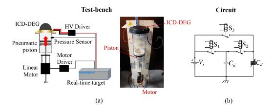
**Figure 3.** (a) Schematic and photograph of the experimental setup. (b) Schematic of the control circuit. In the picture,  $V_s$  is the supply voltage,  $C_d$  is the variable DEG capacitance,  $C_a$  is the in-parallel capacitance, and  $S_1$ ,  $S_2$ ,  $S_3$  denote the switches. HV: high-voltage; ICD-DEG:inflated circular diaphragm DEG.
