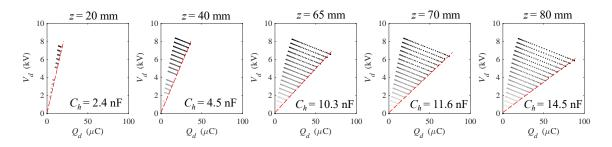
**Figure 5.** Generation cycles on the Q - V plane and indication of the evaluated capacitance  $C_h$  of the inflated DEG during the priming phase. Note that the value of the DEG capacitance in the flat configuration was measured with the same procedure at z = 0 and resulted in  $C_l = 1.9$  nF. Some tests at intermediate voltages are missing for piston displacements of 20 mm and 40 mm due to a few faults in the data acquisition.
