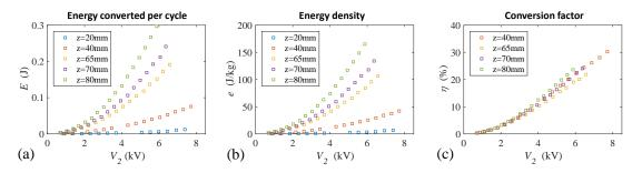
**Figure 6.** Figures of merit for different inflation levels (calculated as the average over four cycles) plotted against the priming voltage: (a) Converted energy; (b) Energy density; (c) Conversion factor (values for z = 20 mm are not reported since the relative small amount of the energy generated makes the estimation unreliable in this case).
