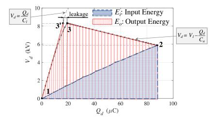
**Figure 4.** Charge voltage Q - V plot of a sample generation cycle. It is worth noting that only the states **2** and **3'** are actual physical states of the DEG, while **3** is a point such that  $V_3 = V_{3'}$  and  $Q_3 = Q_2 - C_a(V_3 - V_2)$ . The points **3** and **3'** coincide in the case of the absence of charge leaks during the generation phase.
