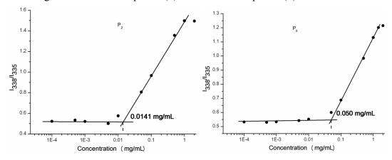
Figure S4 Variation of the intensity ratio ( $I_{338}/I_{335}$ ) as a function of  $P_2$  and  $P_3$  concentrations, the dotted line shows the CMC value.
