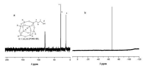
Figure S3 <sup>13</sup>C NMR spectra (a) and <sup>29</sup>Si NMR spectra (b) of POSS-SH
