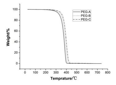
Figure S5 TGA curves of PEG-A, PEG-B, and PEG-C (in N<sub>2</sub>)
