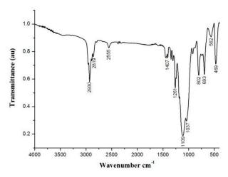
Figure S1 The infrared spectrum of POSS-SH
