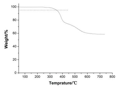
Figure S6 TGA curve of **POSS-SH** (in N<sub>2</sub>)
