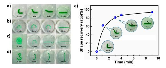
**Figure S4.** (a)–(d) The shape recovery procedures of PAAm-CS hydrogels with different temporary shapes in deionized water; (e) The shape recovery ratio as a function of time in deionized water.
