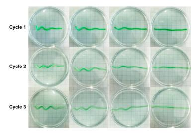
**Figure S9.** Cycled multiple shape memory behavior of the PAAm-CS hydrogel via CS chainentanglement crosslink interaction. Saturated NaCl solution and deionized water were used for shape memory and shape recovery procedures, respectively.
