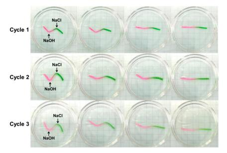
**Firgure S11.** Cycled triple shape memory behavior of the PAAm-CS hydrogel. The straight stripe of hydrogel was dyed in pink and green at the ends. The pink end of the temporary shape was fixed by NaOH solution (75 mM) with 1min and the green end was fixed by saturated NaCl within 2 min. When the hydrogel stripe was immersed in the HCl solution (100 mM), the temporary shape could be recovered to its original shape.
