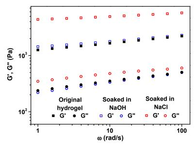
**Figure S2.** Storage modulus (G') and loss modulus (G'') of original PAAm-CS hydrogel and hydrogels soaked in NaOH or NaCl solution, respectively.
