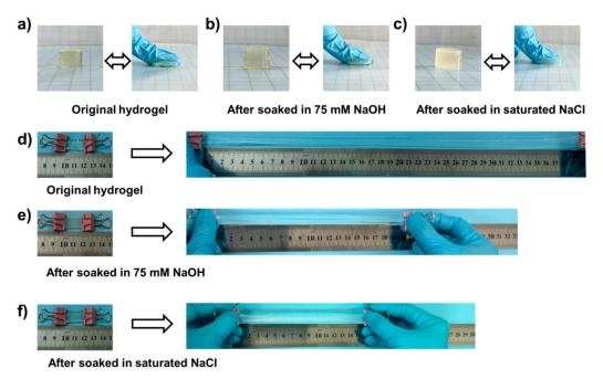
Figure S1. The mechanical properties of different hydrogels. (a)–(c) Photographs of finger compression; (d)–(f) Photographs of stretched hydrogels.
