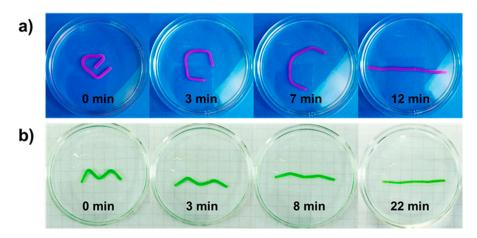
**Figure S7.** The recovery procedures of the PAAm-CS hydrogel with different stimuli. (a) The temporary shape was fixed by CS physical microcrystal crosslink interaction and the shape recovery is induced by HCl (100 mM); (b) The temporary shape was fixed by CS chain-entanglement crosslink interaction and the shape recovery is carried out in deionized water.
