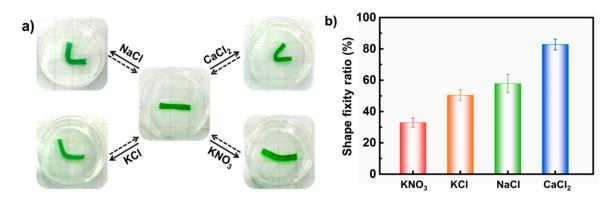
**Figure S5.** (a) The shape memory behavior based on the CS chain-entanglement induced by various saturated saline solutions. All the dashed lines indicate the temporary shape hydrogel will be recovered in the deionized water; (b) The shape fixity ratios based on the CS chain-entanglement as a function of saturated saline solutions.
