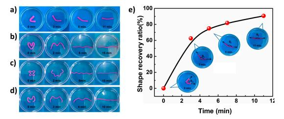
**Figure S3.** (a)–(d) The shape recovery procedures of PAAm-CS hydrogels with different temporary shapes in 100 mM HCl; (e) The shape recovery ratio as a function of time in 100 mM HCl.
