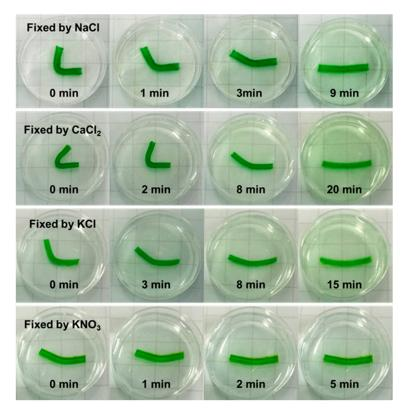
**Figure S6.** The recovery processes of the PAAm-CS hydrogel in deionized water, in which the temporary shapes are fixed by different saturated salt solutions.
