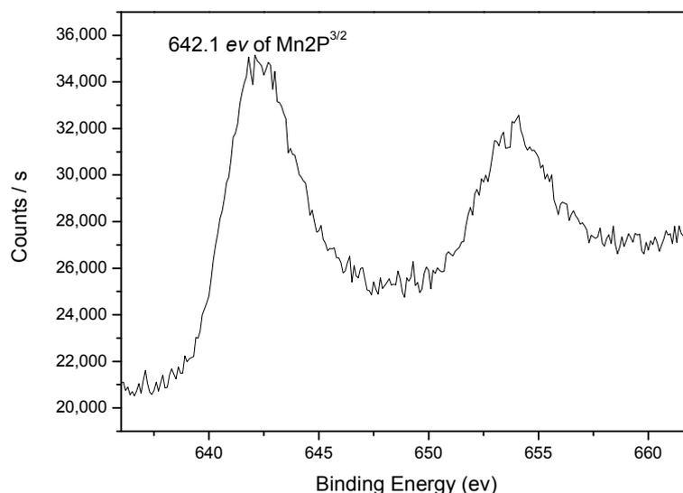
**Figure 5.** XPS spectra of catalyst 1.
