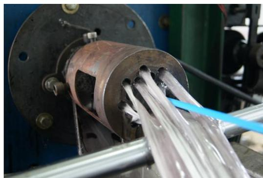
**Figure 6.** Tube insertion for hollow section.
