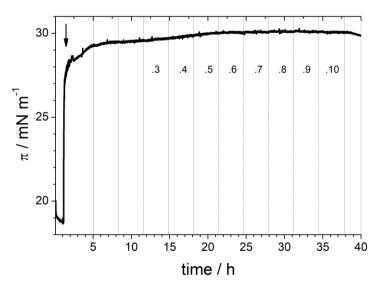
**Figure S8.** Time-course of adsorption of Sar1 (100 nM) to an MMM monolayer spread on a  $D_2O/HKM$  buffer subphase in the presence of GMP-PNP (2  $\mu$ M). The numbers in the figure denote the number of the cycle of the IRRA spectra recordings that were included in the analysis.
