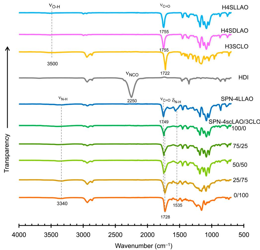
**Figure S5.** FT-IR spectra of H4SLLAO, H4SDLAO, H3SCLO, HDI, SPN-4LLAO and SPN-4scLAO/3CLOs (100/0, 75/25, 50/50, 25/75 and 0/100).
