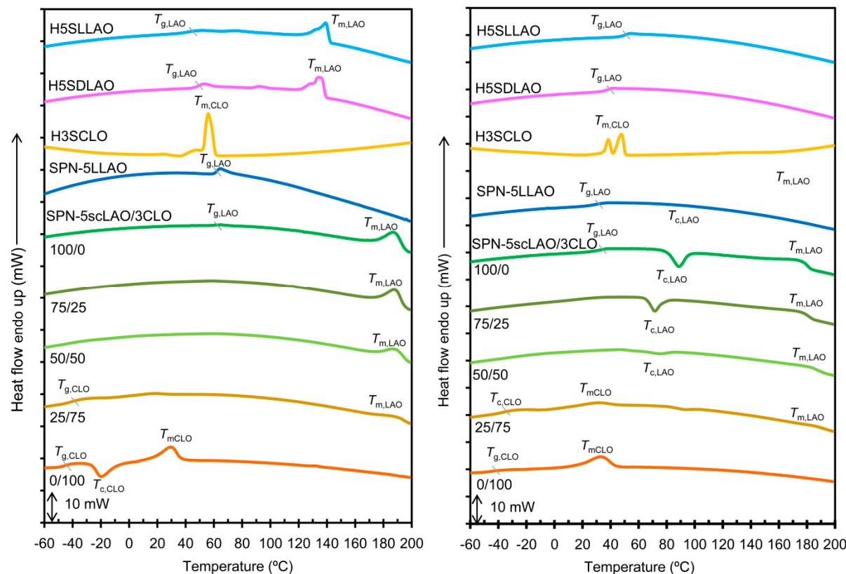
**Figure S9.** The first and second heating DSC curves for H5SLLAO, H5SDLAO, H3SCLO, SPN-5LLAO and SPN-5scLAO/3CLOs (100/0, 75/25, 50/50, 25/75 and 0/100).
