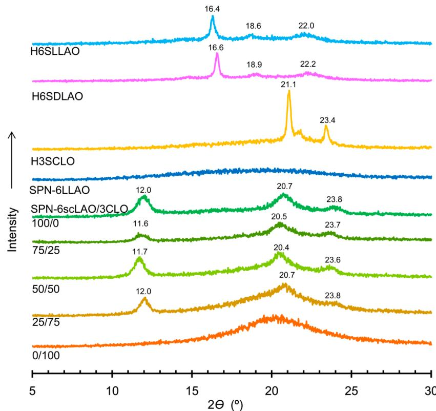
**Figure S8.** XRD patterns of H6SLLAO, H6SDLAO, H3SCLO, SPN-6LLAO and SPN-6scLAO/3CLOs (100/0, 75/25, 50/50, 25/75 and 0/100).
