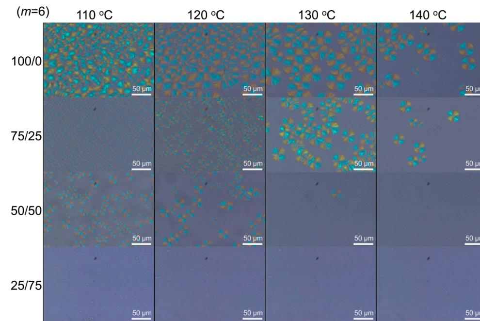
**Figure S11.** Polarized optical microscope images of the SPN-6scLAO/CLOs 100/0, 75/25, 50/50 and 25/75 held at a specified temperature for 10 min after melted at 220 °C.
