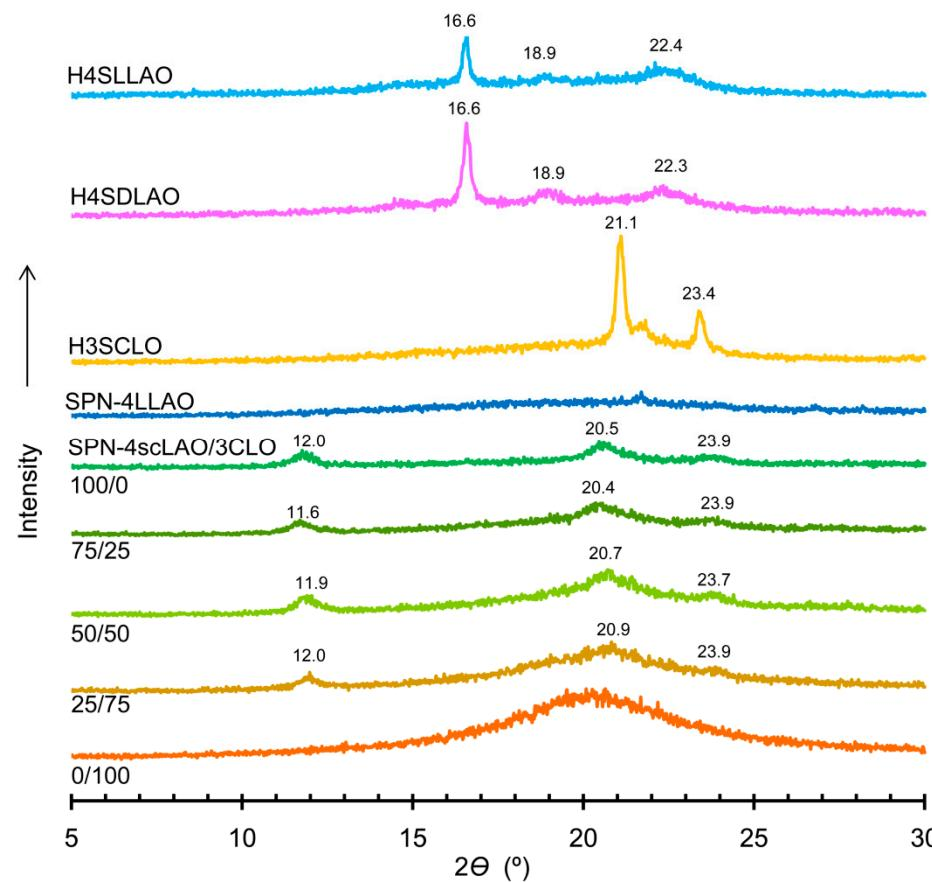
**Figure S7.** XRD patterns of H4SLLAO, H4SDLAO, H3SCLO, SPN-4LLAO and SPN-4scLАО/3CLOs (100/0, 75/25, 50/50, 25/75 and 0/100).
