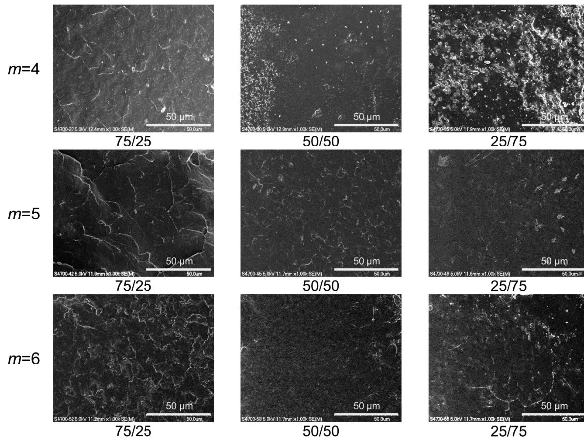
**Figure S12.** FE-SEM images of the fractured surfaces of SPN-mscLAO/3CLO 75/25-25/75 conetworks ( $m = 4, 5$  and  $6$ ).
