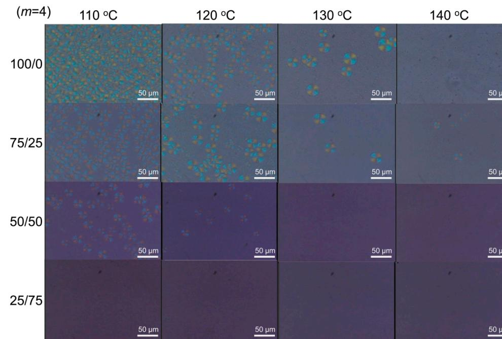
**Figure S10.** Polarized optical microscope images of the SPN-4scLAO/CLOs 100/0, 75/25, 50/50 and 25/75 held at a specified temperature for 10 min after melted at 220 °C.
