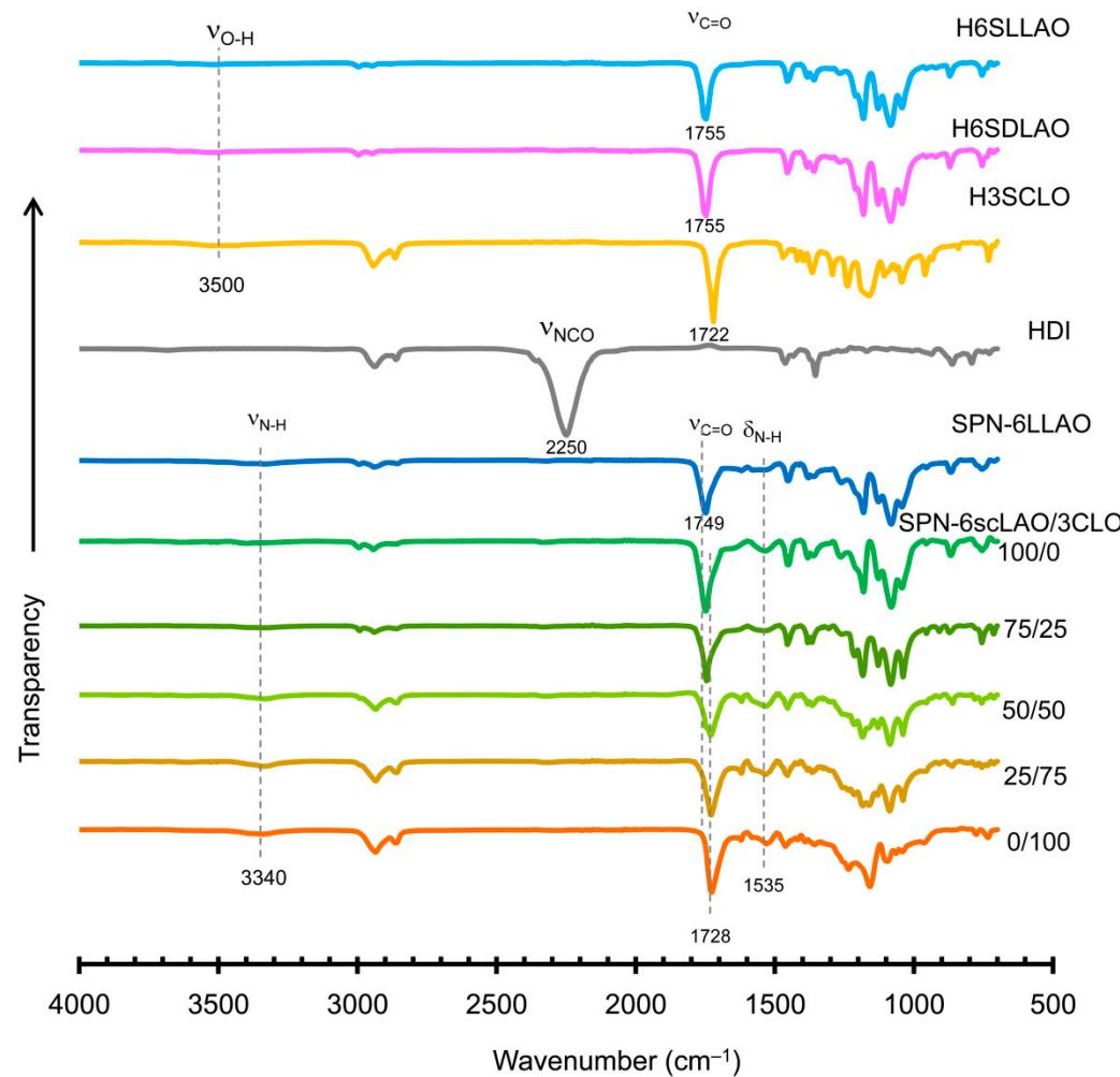
**Figure S6.** FT-IR spectra of H6SLLAO, H6SDLAO, H3SCLO, HDI, SPN-6LLAO and SPN-6scLAO/3CLOs (100/0, 75/25, 50/50, 25/75 and 0/100).
