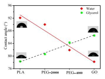
Figure 1. Photographs of contact angles (at 25 °C) and measured contact angles of sole sample.
