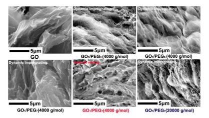
**Figure 2.** Scanning electron microscope (SEM) images of GO and the hybrid GO/PEG composites with different component ratio under different premixing method.
