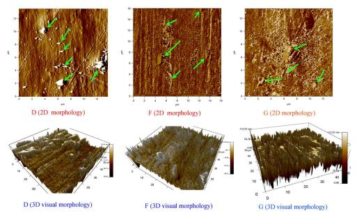
**Figure 3.** 2D grayscale morphologies of (D) GO<sub>1</sub>/PEG<sub>3</sub>/PLA<sub>96</sub> and (F) GO<sub>1</sub>/PEG<sub>7</sub>/PLA<sub>92</sub> based on dynamic impregnating, (G) GO<sub>1</sub>/PEG<sub>7</sub>/PLA<sub>92</sub> based on internal mixing and corresponding 3D visual morphologies obtained using AFM.
