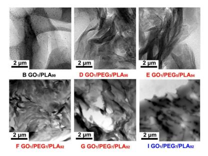
**Figure 4.** Transmission electron microscopy (TEM) images of GO/PLA and GO/PEG/PLA multi-phase composites with the introduction of GO/PEG of different component ratios under different melt-compounding.
