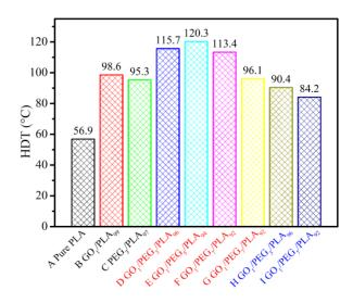
**Figure 10.** HDT of pure PLA, GO/PLA, PEG/PLA, and GO/PEG/PLA multi-phase composites in the case of different component ratio.
