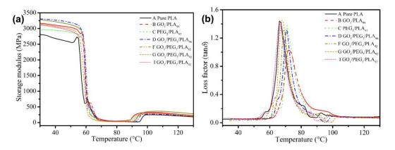
**Figure 9.** DMA curves of pure PLA, GO/PLA, PEG/PLA, and GO/PEG/PLA multi-phase composites in the case of different component ratio. (**a**) Storage modulus curves; (**b**) loss factor curves.
