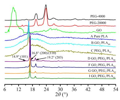
**Figure 6.** Wide angle X-ray diffraction (WAXD) diffraction patterns of PEG, pure PLA, GO/PLA, PEG/PLA, and GO/PEG/PLA multi-phase composites with different component ratio under different melt-compounding.
