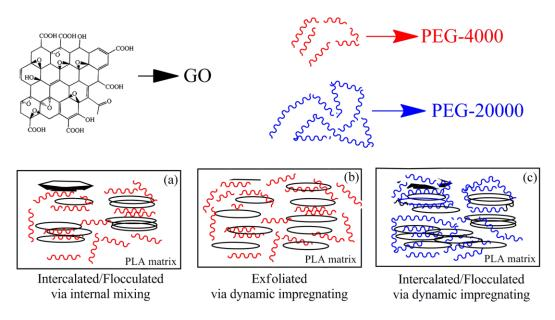
**Figure 11.** Physical model for dispersed morphologies of GO/PEG in PLA matrix with different molecular weight via dynamic impregnating and/or internal mixing, respectively. (**a**) represents GO/PEG-4000/PLA nanocomposite via internal mixing, (**b**) represents GO/PEG-4000/PLA nanocomposite via dynamic impregnating and (**c**) represents GO/PEG-20000/PLA nanocomposite via dynamic impregnating.
