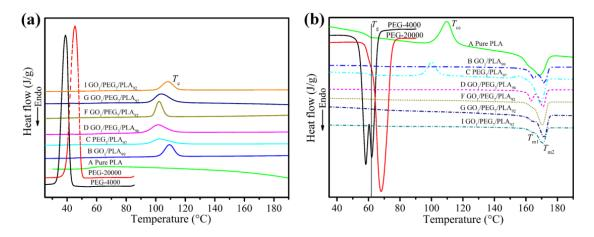
**Figure 7.** Differential scanning calorimetry (DSC) curves of PEG, pure PLA, GO/PLA, PEG/PLA, and GO/PEG/PLA multi-phase composites with different component ratio under different melt-compounding. (a) Cooling curves; (b) melting curves.
