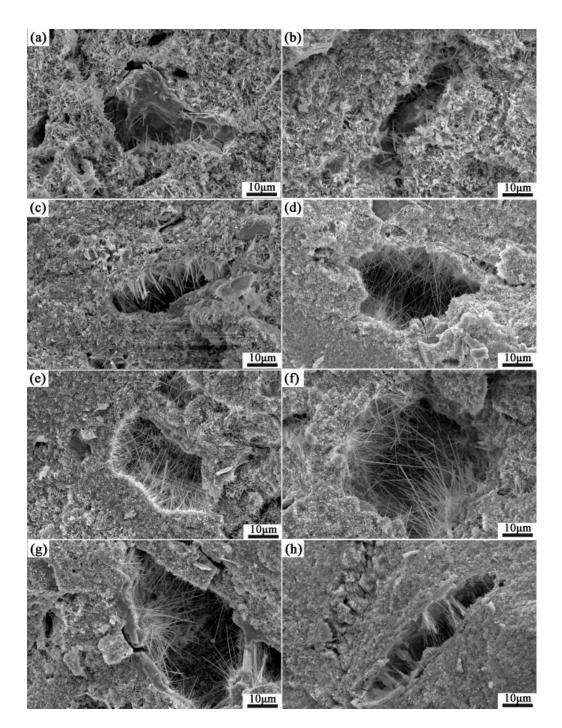
**Figure 3.** SEM images of the fracture surface of (**a**) MOC-3 adhesive; (**b**) MOC-4 adhesive; (**c**) MOC-5 adhesive; (**d**) MOC-6 adhesive; (**e**) MOC-7 adhesive; (**f**) MOC-8 adhesive; (**g**) MOC-9 adhesive; (**h**) MOC-10 adhesive.
