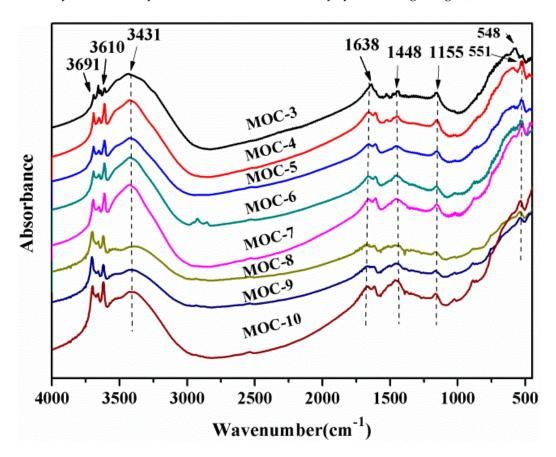
Figure 1. Fourier Transform Infrared (FTIR) spectra of MOC adhesives.
