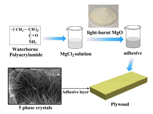
Scheme 1. Schematic illustration of plywood bonded with inorganic adhesives.
