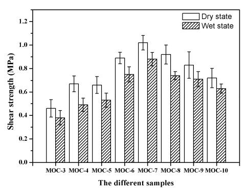
Figure 6. The shear strength of plywood bonded by the MOC adhesives.
