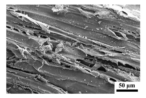
Figure 4. SEM micrograph of the fracture surface of the wood surface bonded by the MOC-7 adhesive.
