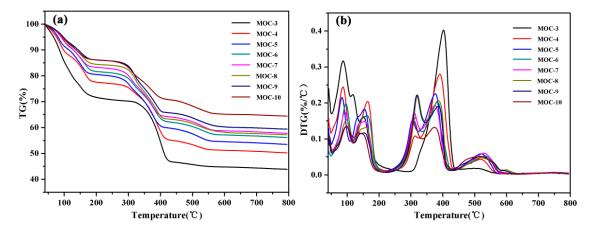
**Figure 5.** The (**a**) thermogravimetric (TG); and (**b**) derivative thermogravimetric (DTG) curves of the MOC adhesives.
