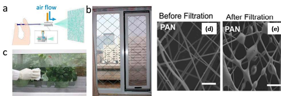
**Figure 13.** Real window based PM filtering performances. (a) Practical model of the blowspinning setup for window screen coating; (b) Real window coated with PAN-NFs; (c) Successful wiping of nanofibers from the window screen with a tissue paper and SEM images of PAN-NFs (d) before and (e) after filtration.
