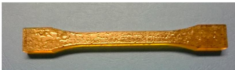
**Figure 3.** Specimens of the cured adhesive after 7 days of curing.
