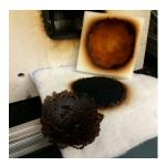
Figure 3. Digital image of char removed from the FPUF tested with BF-2.
