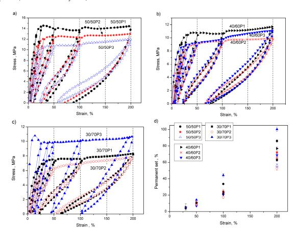
**Figure 7.** Stress–strain curves from cyclic tensile tests obtained for: (a) PTT-*b*-PEOT 50/5; (b) PTT-*b*-PEOT 40/60 and (c) PTT-*b*-PEOT 30/70 with PEG molecular weights of 1000, 2000 and 3000 g/mol and (d) permanent set of specimens in tension direction resultant from maximum attained strain in the cyclic deformation for PTT-*b*-PEOT copolymers.
