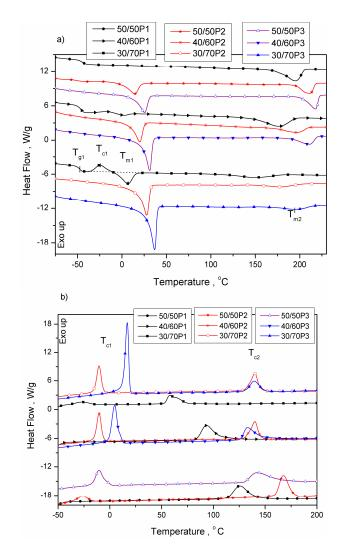
**Figure 2.** DSC thermograms obtained during 2nd heating (**a**) and cooling (**b**) for PTT-*b*-PEOT copolymers.
