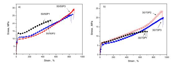
**Figure 6.** Representative stress–strain curves for PTT-*b*-PEOT copolymers containing 50 (**a**) and 70 (**b**) wt % of PEOT flexible segments.
