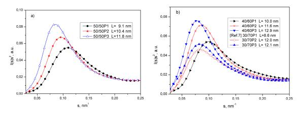
**Figure 5.** The Lorentz–corrected SAXS patterns at 23 °C (L—long period) for PTT/PEOT ratio of (**a**) 50/50 and (**b**) 40/60 and 30/70.
