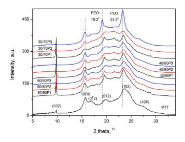
Figure 4. WAXS patterns of PTT homopolymer and PTT-b-PEOT copolymers at 23 °C.
