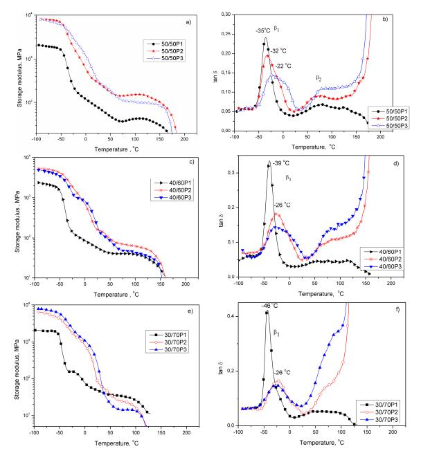
**Figure 3.** The storage modulus (**a**,**c**,**e**) and tan  $\delta$  (**b**,**d**,**f**) as a function of temperature for PTT-*b*-PEOT copolymers with PEOT content of 50 (**a**,**b**), 60 (**c**,**d**) and 70 (**e**,**f**) wt %.
